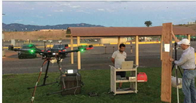
Figure 1. First outdoor laser UAV testing for measuring contact-free, reference-free displacements (Albuquerque, New Mexico).
