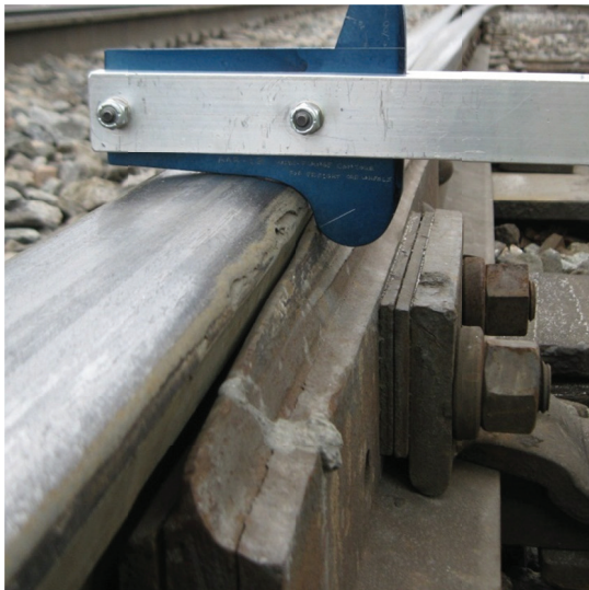
Unsafe wheel-rail contact as determined by TGAAR1B Gauge with contact below the 60° mark.
