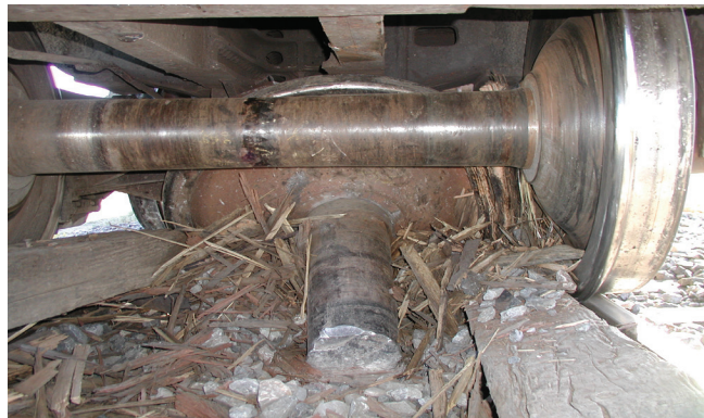
Figure 1: Broken railroad axle
