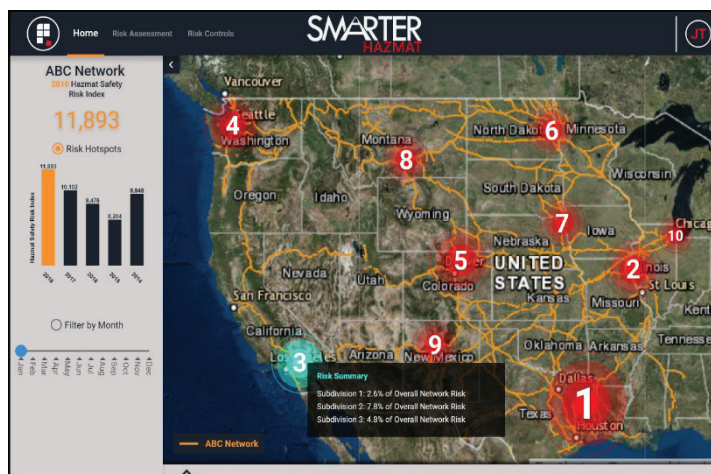
Figure 2. Snapshot of prototype design showing subdivisions and areas in an example network that may pose an elevated risk (hypothetical data shown). The prototype also allows exploration of some risk reduction strategies and their effect on overall- and location-based safety risk. Additionally, potential risk accumulation from future or planned hazmat movements are planned to be analyzed through the prototype system.
