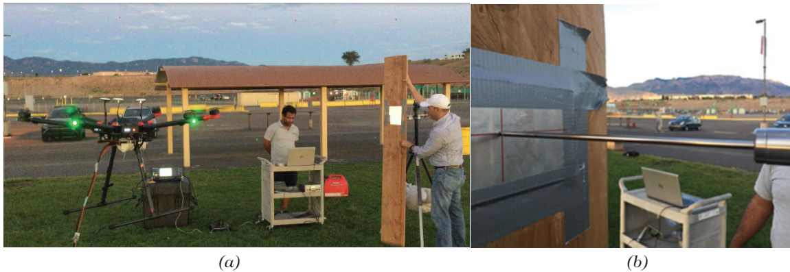
Figure 1: First outdoor laser UAV testing for measuring contact-free, reference-free displacements compared with reference displacements: (a) experiment general view; (b) reference displacement detailed view.
