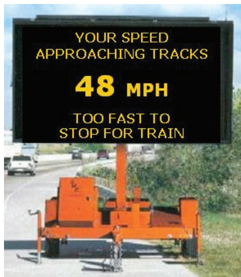
Figure 1: Conceptual example of a driver feedback display for passive grade crossings
