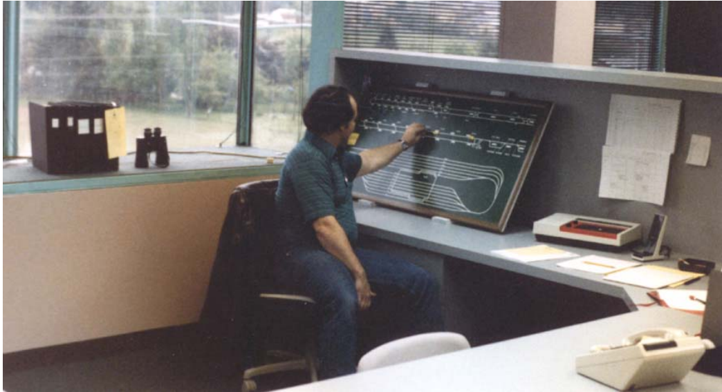
FIGURE 2 Essential tools for yard operations: magnet board, telephone, two-way radio, and binoculars.
