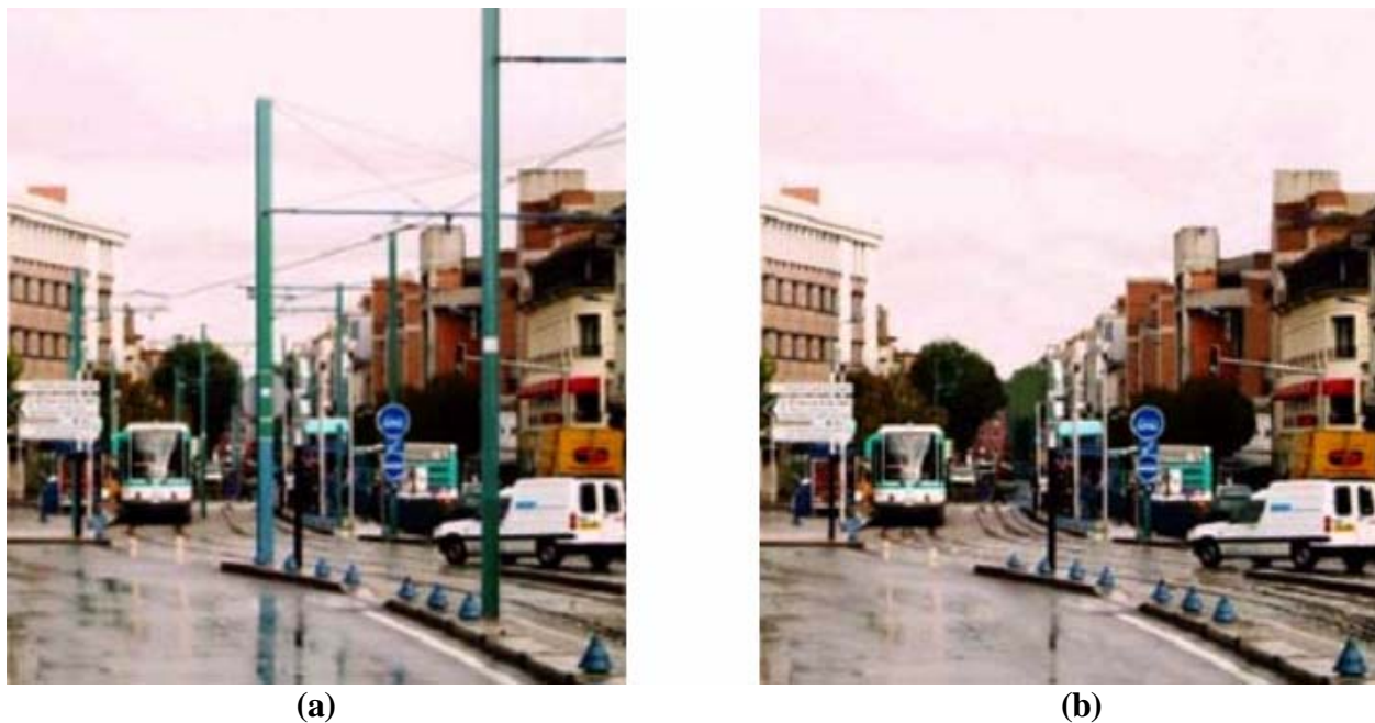
FIGURE 1 Urban landscape (a) with OCS wires; and (b) without OCS wires.
