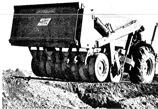
MULTIPLE COMPACTOR —Versatile self-propelled rig combines rubber and steel rolling. Vibration can be added.
