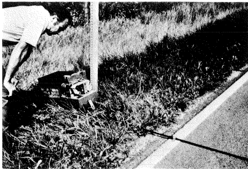
Fig. 22. Twice-a-day service is essential. A service check is an inspection of the counter mechanism to determine that the correct time and count are being recorded.
