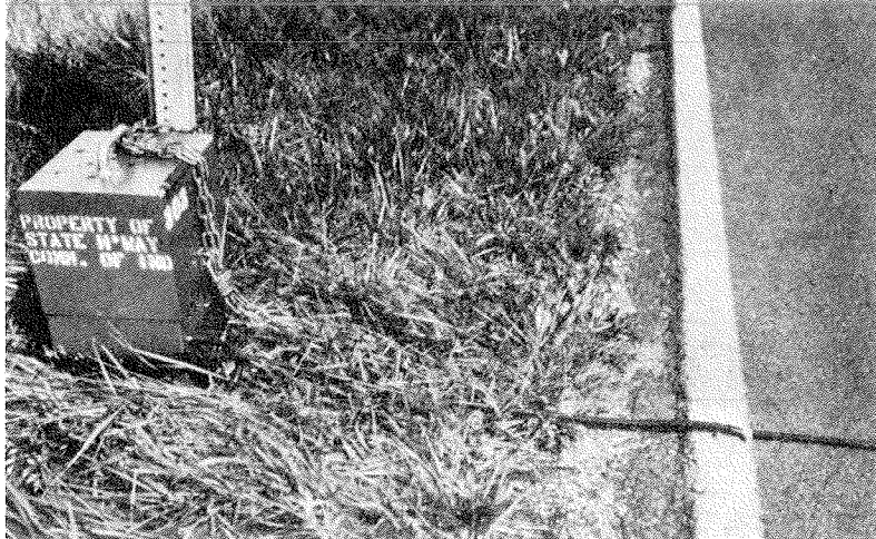
Fig. 13. Counters must be chained and locked in an upright position to a tree, sign post or utility pole. Chain must be snug so counter cannot tip over.
