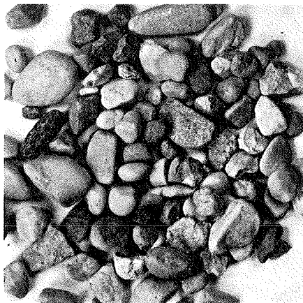
Fig. 13. This is also a poorly-graded gravel. Since several sizes are missing, to qualify as a well-graded gravel, the material is also called a gap-graded gravel. As a base, it would be more stable than the uniformly-graded gravel but less stable than the well-graded gravel.
