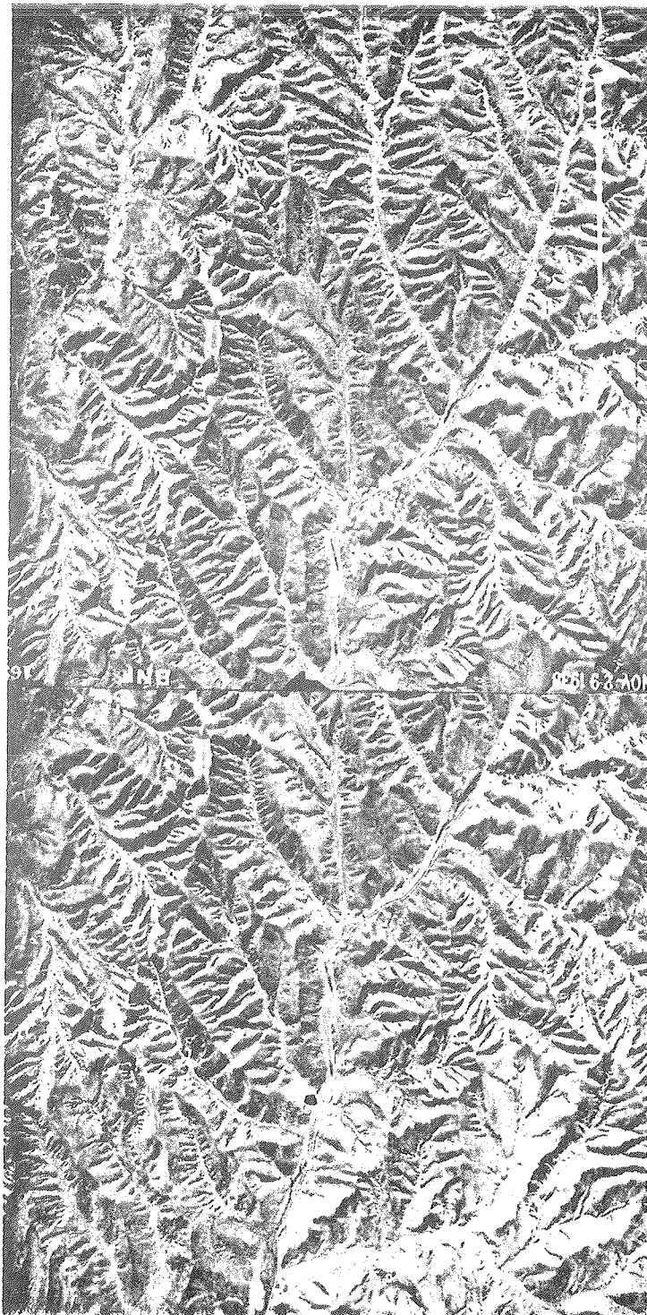
Figure 60. Loess, Lincoln County, Nebr. This stereo pair shows loess of great depth which is identified by steep-sided, flat-bottomed gullies, equal slopes in hills and valleys, and soft tones. The catsteps — small slumps — are seen as light fine contours all over the area. (Aerial photograph by U. S. Department of Agriculture)
