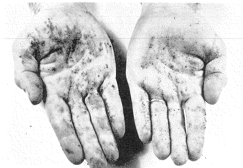
Fig. 10. In the hand stain test, wet or thoroughly damp coarse-grained soils may be determined to be clean or dirty. Dirty material, after being firmly squeezed in the hand, leaves a stain or discoloration—as on the left. A clean material leaves essentially no stain—as on the right.
