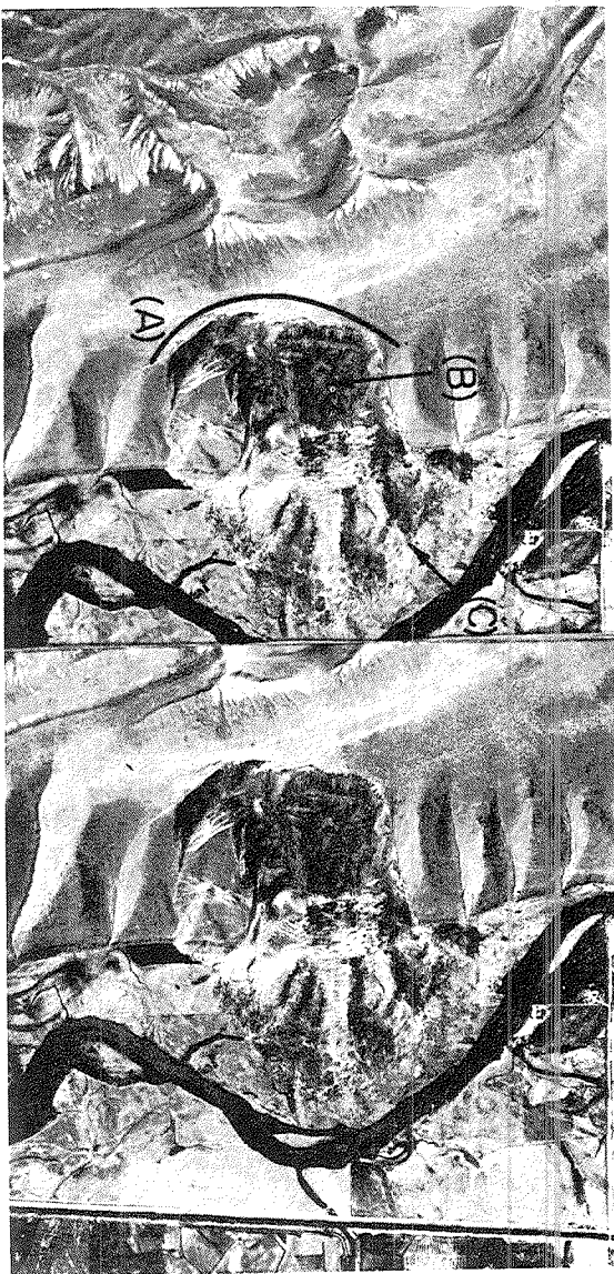
Figure 4.—Stereogram showing typical characteristics of a landslide on aerial photographs: Semicircular scarp (A); depression (B); and hummocky topography (C). Location in Yakima County, Wash. (Courtesy U.S. Department of Agriculture.)
