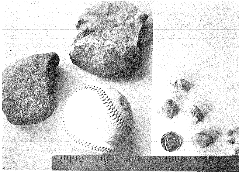
Fig. 1. In the Unified Soil Classification System, gravels are divided only into coarse and fine sizes. Coarse gravel ranges from 3 in. (baseball size) to \frac{3}{4} -in. (about the diameter of a nickel). Fine gravel ranges from below \frac{3}{4} in. to about \frac{1}{4} in.—the size of a dried pea.
