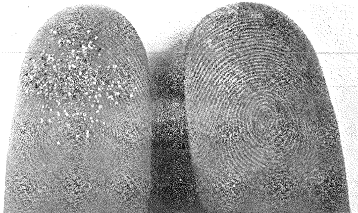
Fig. 3. This photograph shows the size relationship between fine sand and fines (silt and clay particles). Sharp observation of the photograph shows that the silt and clay particles fit down into the crevices of the "finger prints" (right) and that the fine sand particles do not (left). Fine sand feels sharp and gritty while both silt and clay particles feel soft and smooth like flour.
