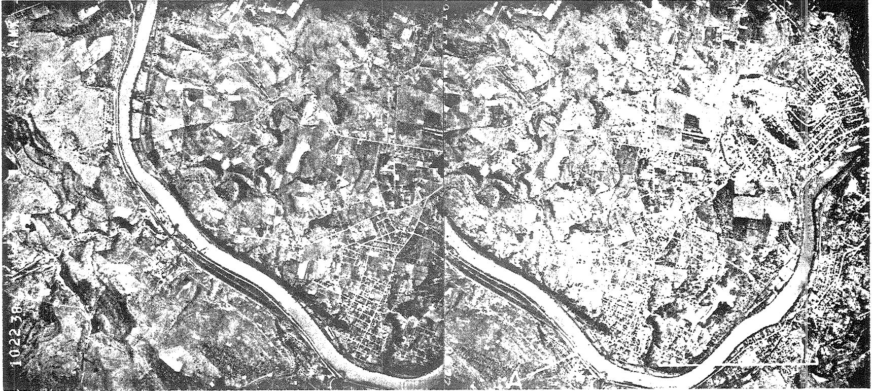
Figure 48. Clay shale, Monongalia County, W. Va. This stereo pair shows an area where clay shales predominate and landslides are active. There are very few competent beds in the general area as evidenced by the rounded, soft slopes and dull, uniform, gray tones. Minor irregularities as signs of movement are seen in most of the steep slopes. Even without artificial disturbances, nature is actively reducing the relief of the area by creeps, flows, and slides. At area (A), both the railroad and highway have experienced continuous landslide troubles. The irregular outline of the bank along the river and the patchwork on the road pavement are clearly seen in the photos. The steep slope and active attack by the river provides a favorable condition for landslides. Furthermore, surface drainage in the back of the slope is blocked by a hill and water is seeping through the hill toward the river. Such a circumstance is conducive to slides.
