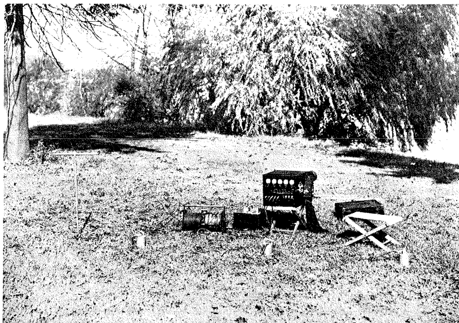
Figure 1. Refraction Seismograph Developed by the Bureau of Public Roads for Use in Shallow Subsurface Explorations
