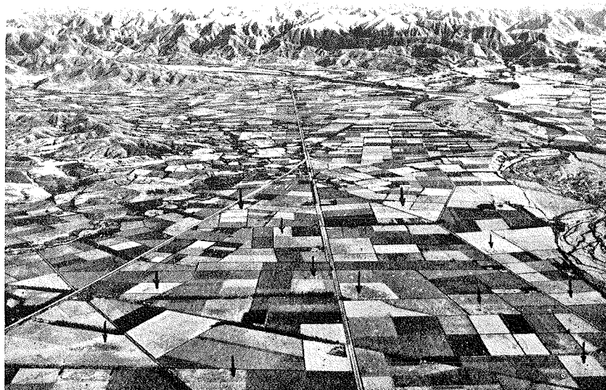
Figure 18. An oblique view of a gravel terrace in New Zealand illustrating the wide application of the major elements of analysis. Not only is the land form apparent but the absence of surface drainage, source of the material, vertical stream banks, and color pattern (arrows) are clearly shown. The checkered field pattern is caused by a variety of crops. Reproduced by permission of New Zealand Aerial Mapping, Ltd.
