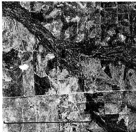
Figure 4. The photograph shows the variation in colors in an area that, from the ground, appears black. Chalk underlies the entire area and where light tones appear the influence of the chalk has modified the silty clay to a No. 9 material. The darkest areas represent Nos. 11 or 12 material. Erosion control in the form of "terracing" is evident. Sheet erosion on these gently sloping areas indicates a condition of retarded internal drainage and implies a clay texture in the subsoil. Bar scale on aerial photographs indicates a distance of one mile.
