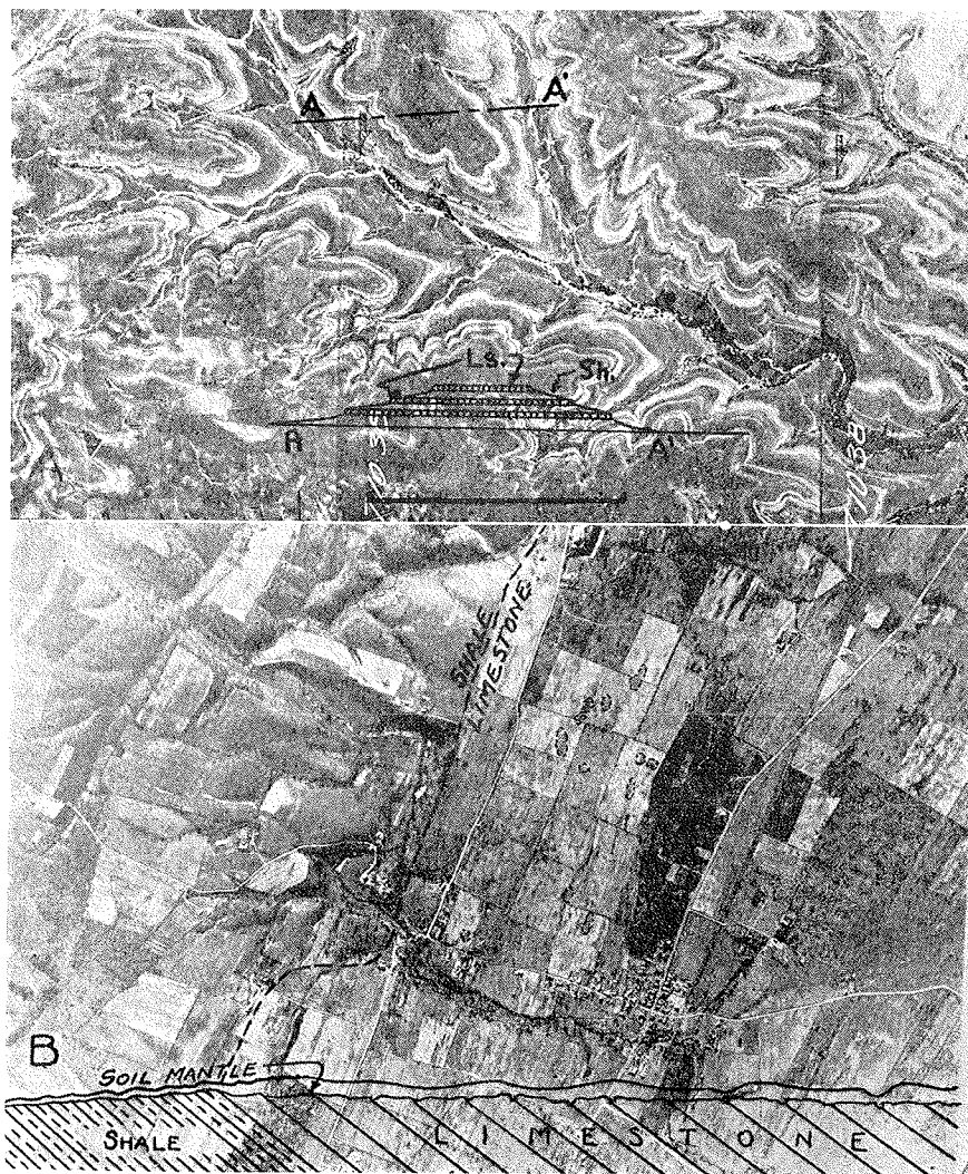
Figure 13. A. Aerial view of nearly horizontal beds of limestone and shale. Geologic erosion has cut through a series of these strata forming a contour-like pattern. In this relatively dry climate the limestone (white) outcrops to form comparatively steep slopes while the soft shale (dark) assumes low, gentle slopes. Sketch on section A-A' illustrates formation. B. Down-dipping beds of shale and limestone form the pattern shown. Shallow impervious soils form on the shale while deep soils mantle the limestone. Note the abrupt change in surface drainage.
