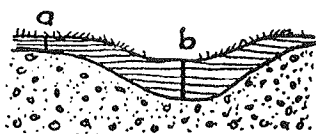
Fig. 34 Open a likely gravel source where overburden is thinnest.
