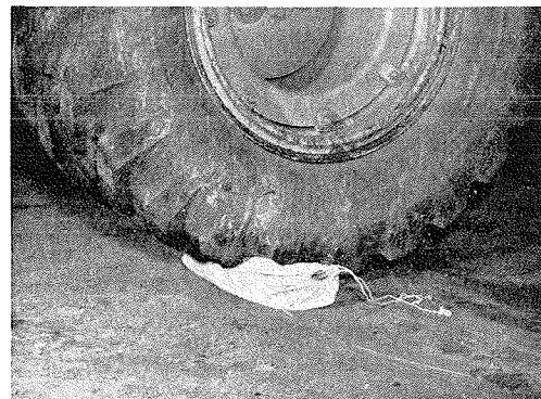
Fig. 41 "Rolling" the quartered sample.
