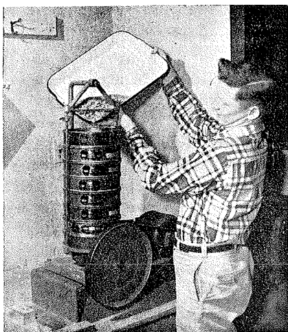
Fig. 42 Using an automatic shaker for sieve analysis.
