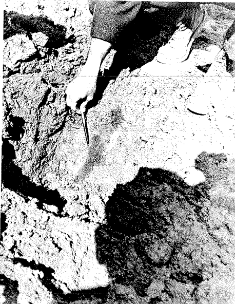
Figure 44. Checking uniformity of mixing with phenolphthalein solution.
