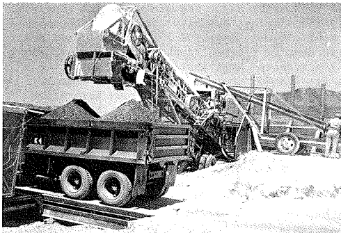
(a) Lime-treated gravel with lime fed by screw conveyor—South Dakota (Ref 21).
