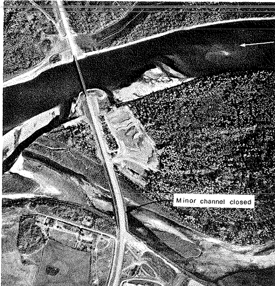
Figure 5.7 Airphoto illustrating the use of a short guide bank on one side only. Note that the construction of a large storage reservoir upstream justified the substantial degree of channel constriction in this case. Note also the sand bars visible through the shallow water.
