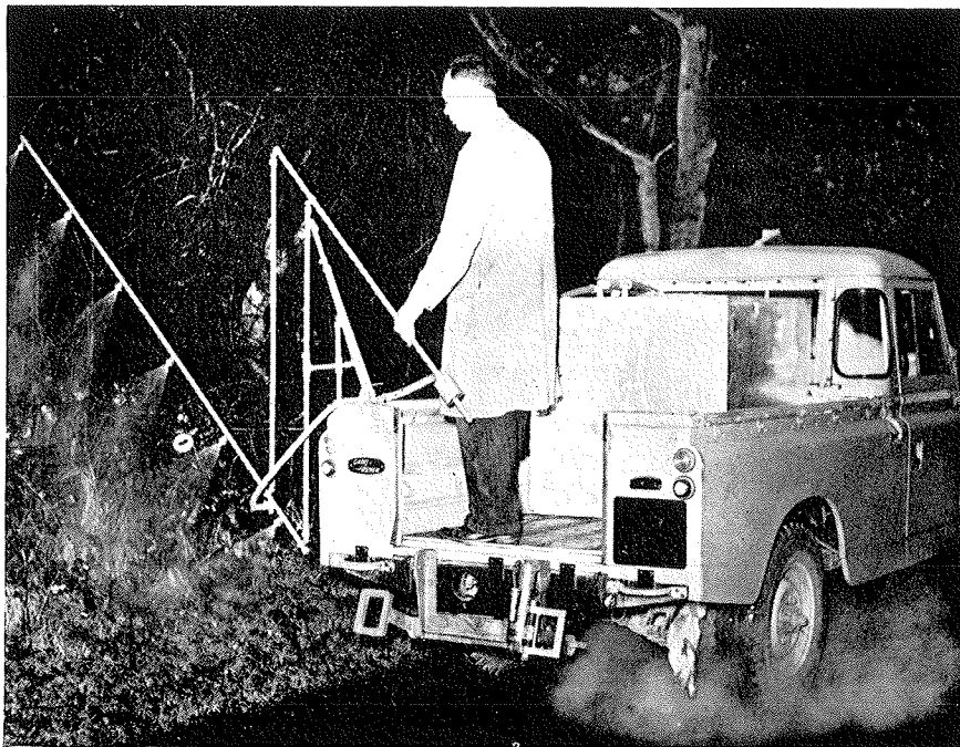
(B) Tank and cantilevered spray bar accessories for a Land Rover, developed for the chemical control of roadside vegetation. The pump is driven from the centre P.T.O., in the cab. ( Photograph—Evers and Wall )
