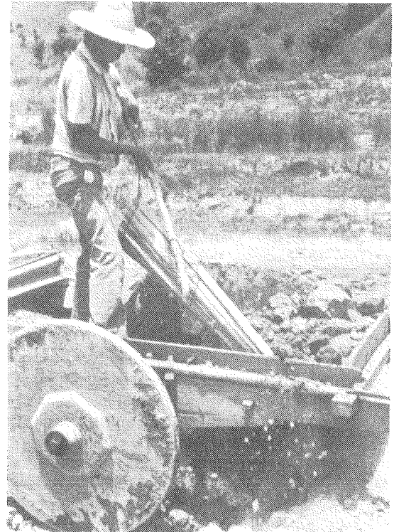
Modified animal-drawn cart: this one has wooden wheels but its bottom consists of bamboo mats which are simply lifted to unload (Philippines)
