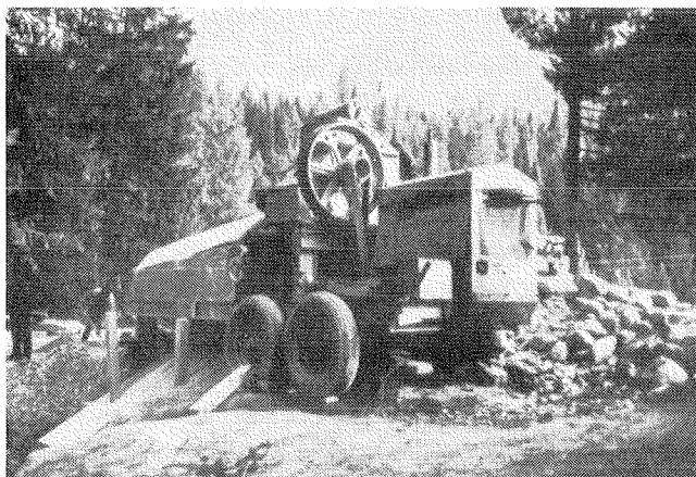
Figure 13. Simple mobile crusher (6-8 tons/h) with integrated screening equipment (11).
