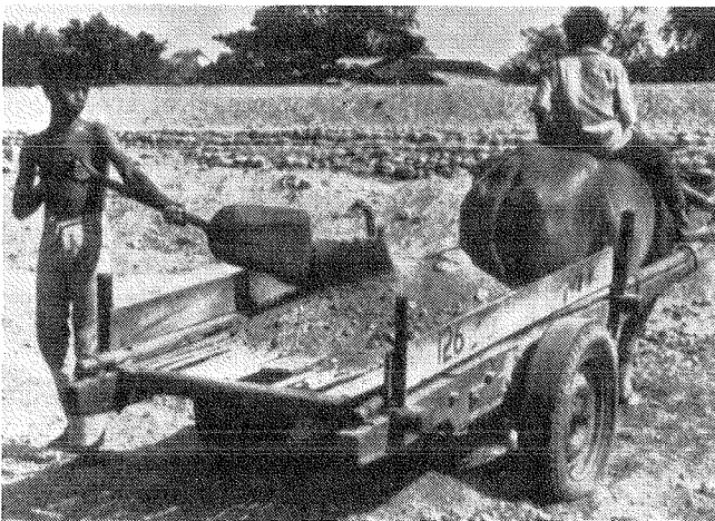
Tractor/trailer combination of small tractor, towed chassis, and hauling container which can be hand-loaded (Southern Africa)
