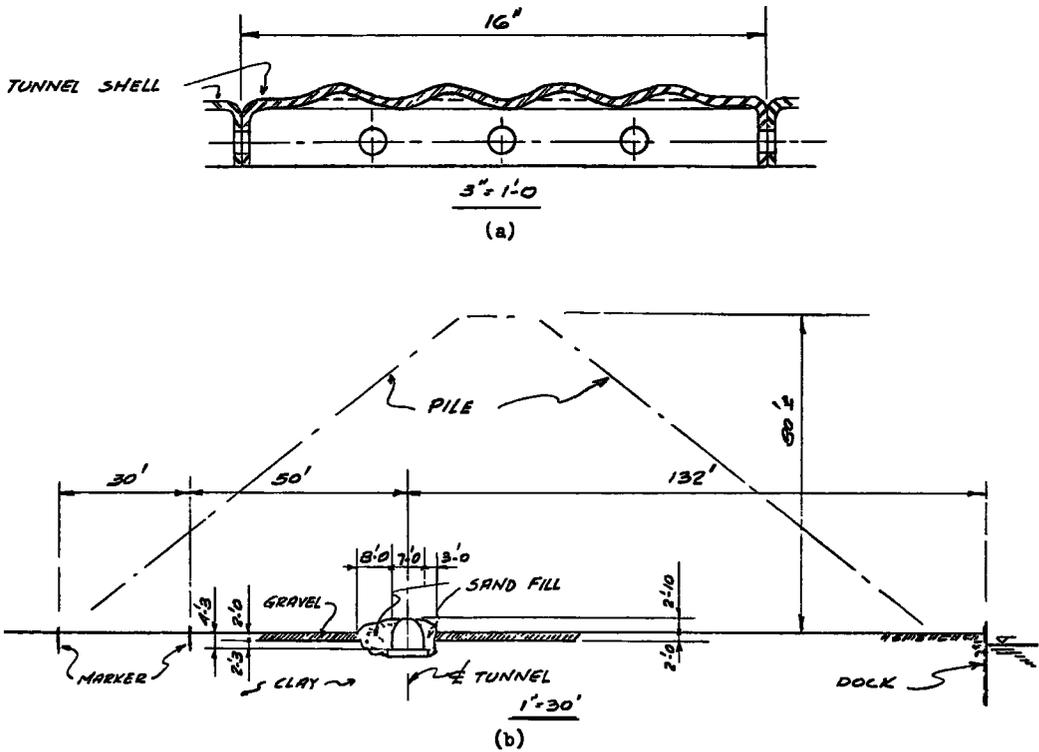
Figure 3. (a) Longitudinal section through liner plate, (b) section through tunnel and maximum size stock pile.
