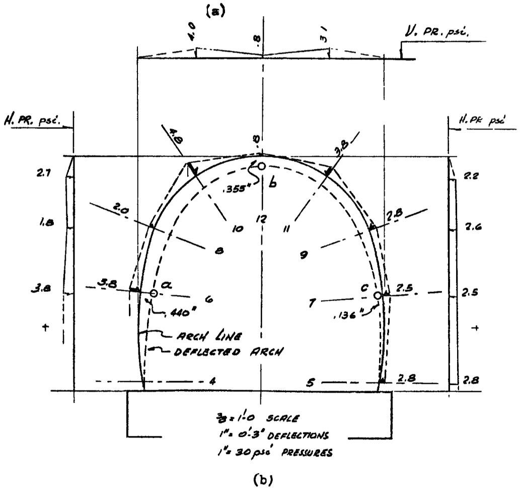
Figure 11. Field measurements 8, (a) loading diagram, (b) gage data.
