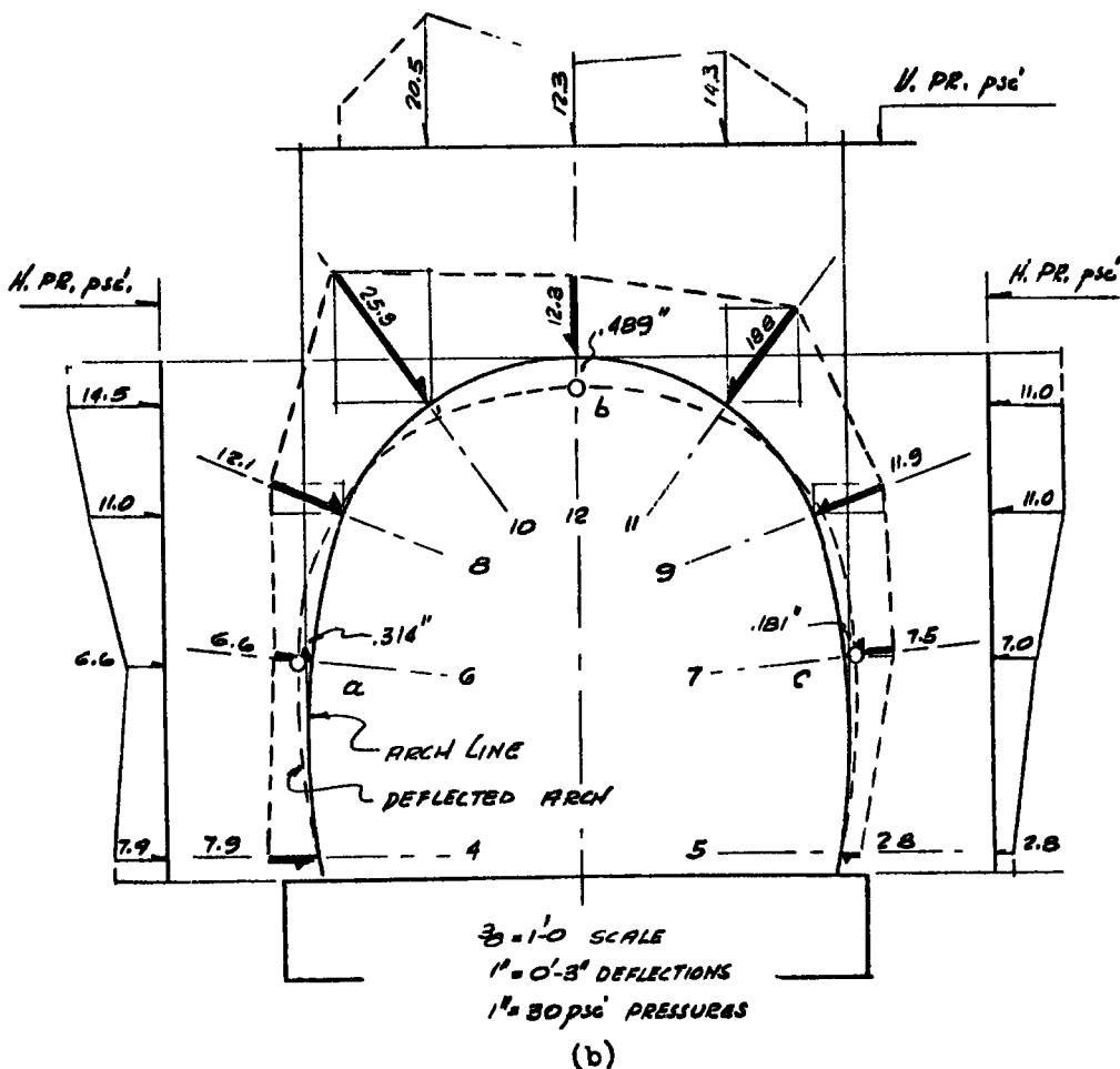
Figure 8. Field measurements 5, (a) loading diagram, (b) gage data.
