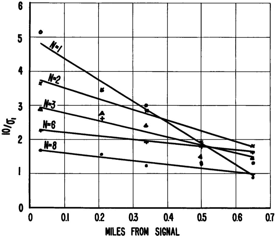
Figure 12.  $10/\sigma_1$  versus distance for nth vehicle.
