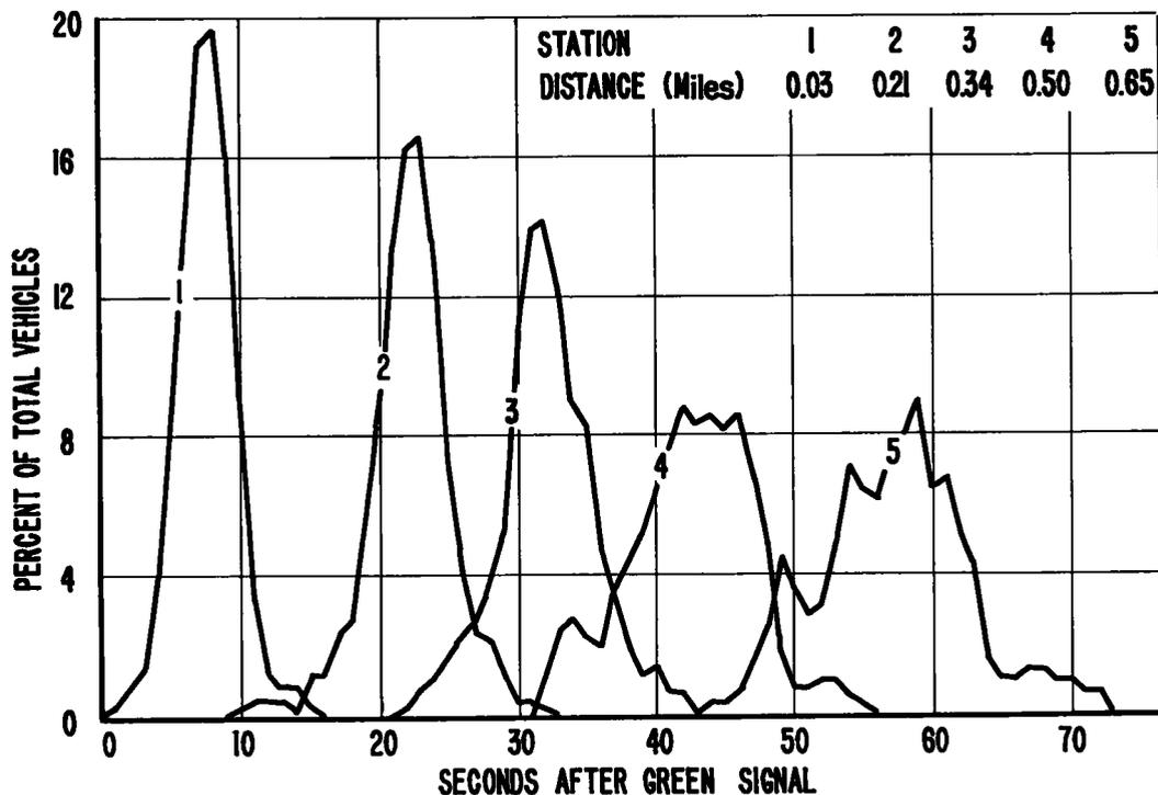
Figure 2. Frequency distributions of arrival times of first vehicle in a platoon at 5 stations distant from the signal.
