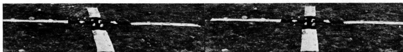
Stereogram 3. Ground view of cross-type target. Materials used are dark red and white muslin. This target is similar to Target No. 2 described in the paper. Its other characteristics are similar to Target No. 1, as illustrated in Stereogram 1 and 2.
