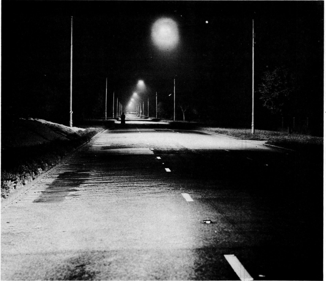
Figure 2. Appearance of the experimental long-spaced lighting system as seen by a driver using his meeting beam (note how the figure, well ahead of the driver's beams, is silhouetted against several bright bands).
