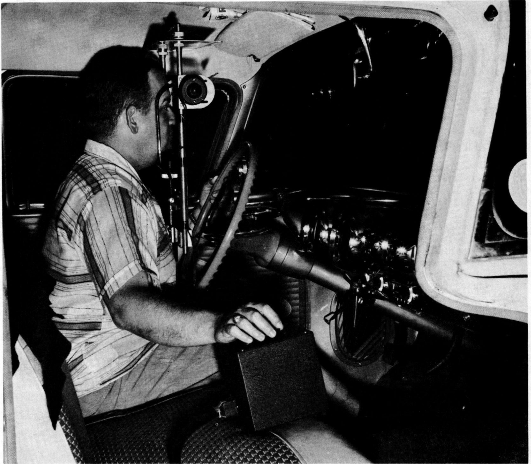
Figure 5. Observer R.K. Drake shows how the Guth evaluator source brightness is remotely controlled from the driver position in an automobile. During the relative visual comfort rating of a roadway lighting system, the shield portion of the headrest assembly is first down steadily for appraisal of the BCD-brightness on his line of sight with luminaires excluded from view. This is followed by automatic rotation of the shield up and down to alternately expose the observer-driver's eyes to the impact sensation judged to be equivalent to the combined brightness of the system luminaires.
