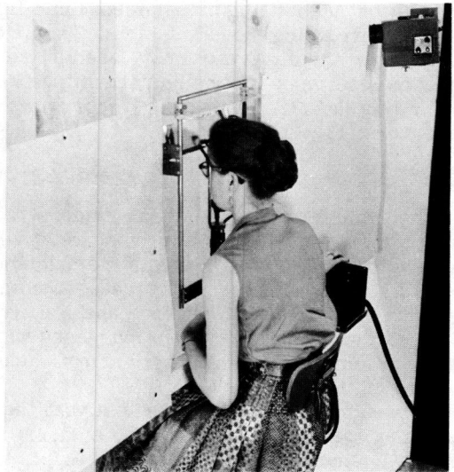
Figure 8. View of observer (center) in the environmental chamber looking at the flashing spot of light (at upper left). Hand control is located to the observer's right, and the brightness meter for making brightness calibrations is at the upper right.
