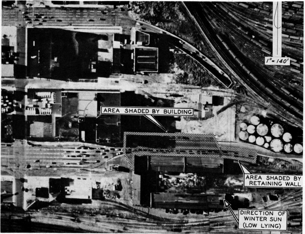
Figure 2. Shadowed entrance ramp.
