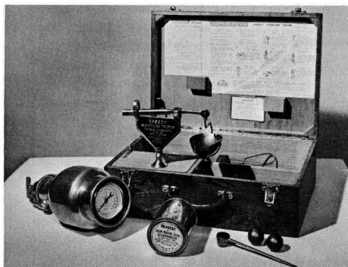
Figure 88. Calcium carbide pressure device for determining moisture content.
