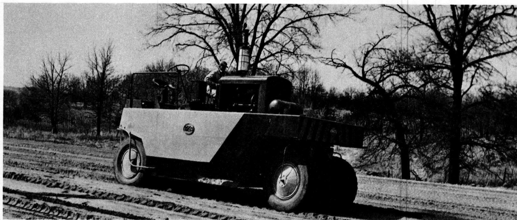
Figure 118. Thirty-ton, 7-wheel, self-propelled pneumatic-tire roller.
