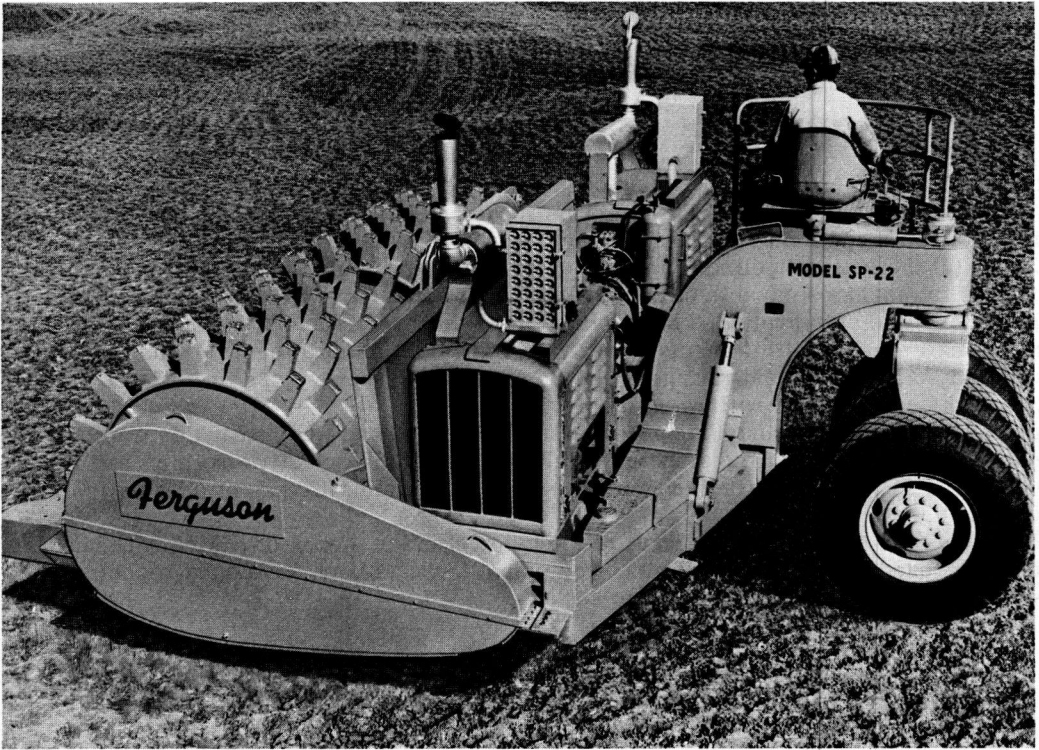
Figure 114. Self-propelled sheepfoot roller having dual drums 60 in. in diameter and 72 in. wide, 144-9.25-in. long tamper feet per drum each having a contact area of 7.5 sq. in. Contact pressures of 656 psi empty (856 loaded with water) and speeds up to 8 MPH.
