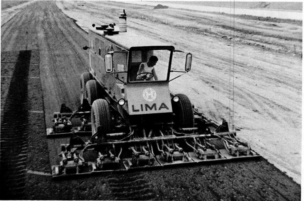
Figure 123. Tandem arrangement of multiple-unit vibrating base-plate compactors for high capacity production.
