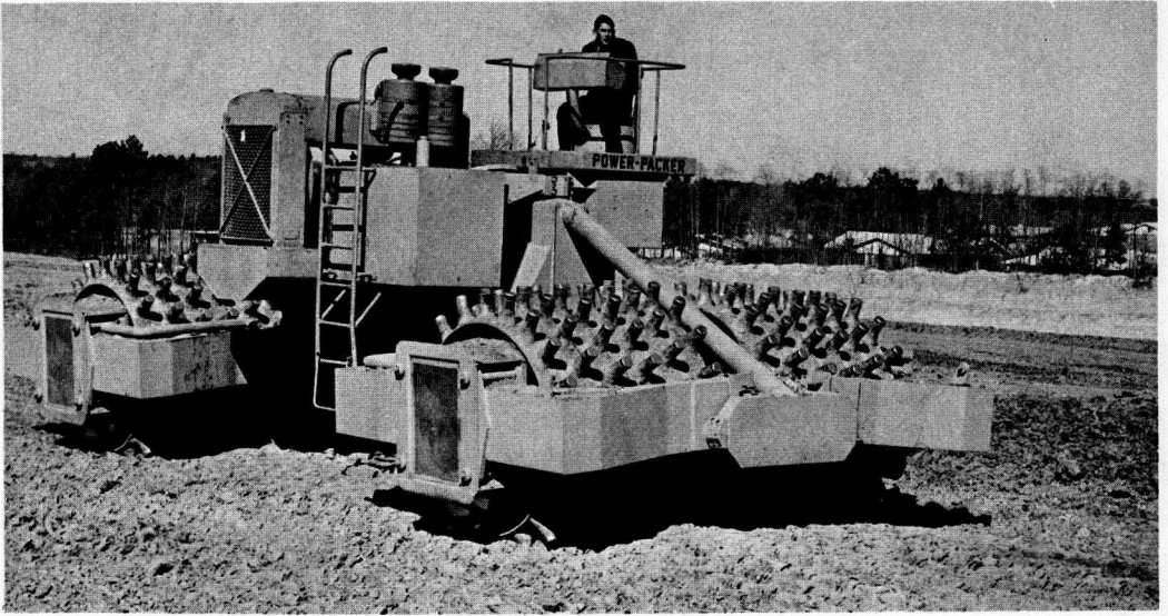
Figure 116. Heavy high-capacity self-propelled sheepfoot roller equipped with four drums each 60 in. wide and 60 in. in diameter, having 120 feet per drum. Tamper feet are 9 in. long and have 10-sq in. end area. Travel speeds up to 5 MPH.
