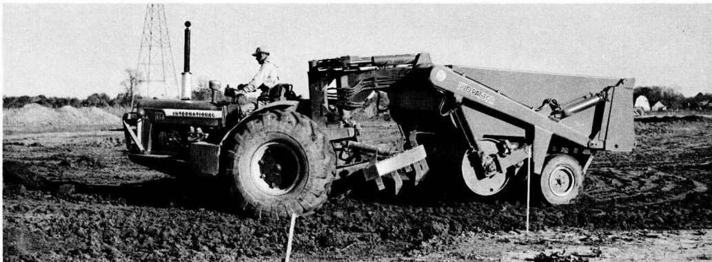
Figure 129. Smooth-wheel and pneumatic-tired rollers combined in one unit. These two types of rollers can be used independently or in combination. Working speeds up to 10 MPH. Tire inflation pressures up to 100 psi. Steel roll can be loaded with loads from 120 to 535 lb per in. of width of roll.
