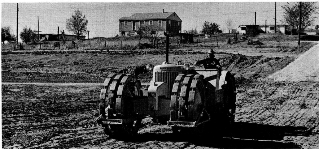
Figure 121. A self-propelled four-wheel-type segmented wheel roller capable of speeds up to 6 MPH.
