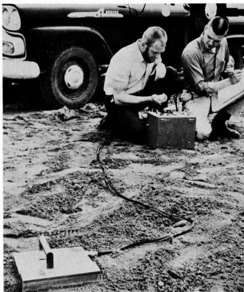
Figure 93. Nuclear surface gage for measuring in-place unit weight (courtesy Michigan State Highway Department).
