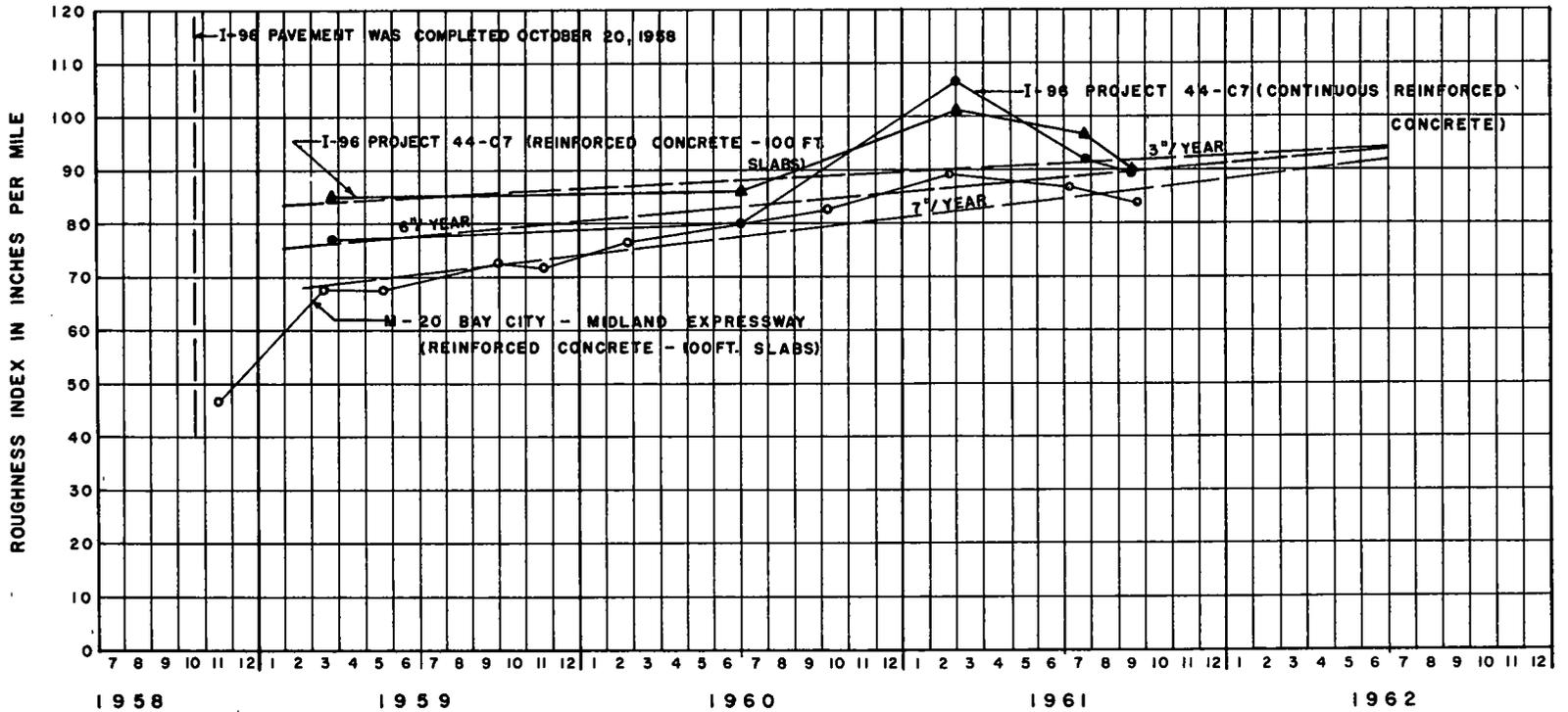
Figure 9. Cumulative change in roughness on specific projects.
