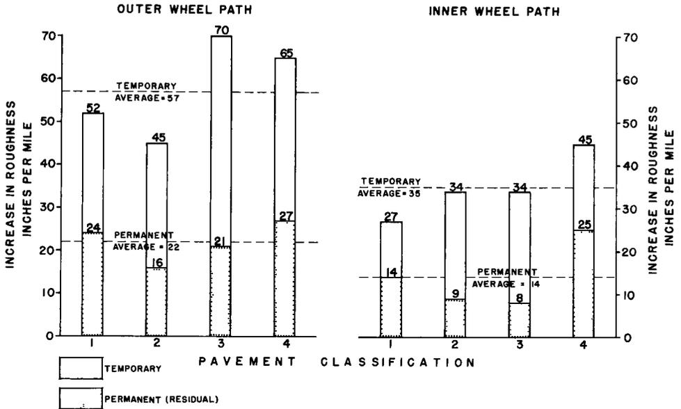
Figure 8. Seasonal fluctuation in pavement profile.
