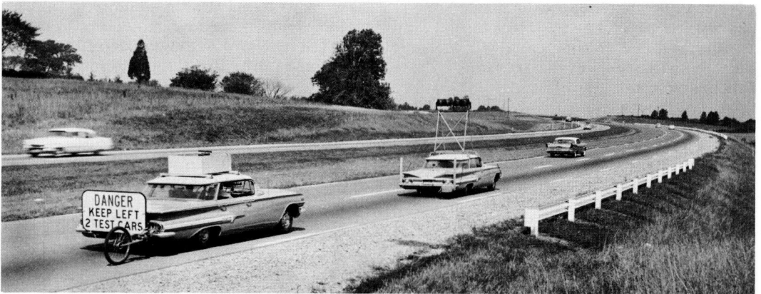
Figure 1. Two-vehicle platoon; lead vehicle with overhead communications system and vertical targets mounted on rear bumper; rear vehicle which had fifth wheel and generator atop car driven by test driver.
