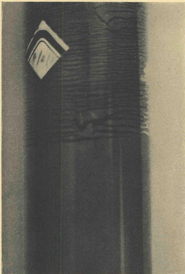
Figure 6. Glass Tube Containing Graded Frozen Silt Specimen
