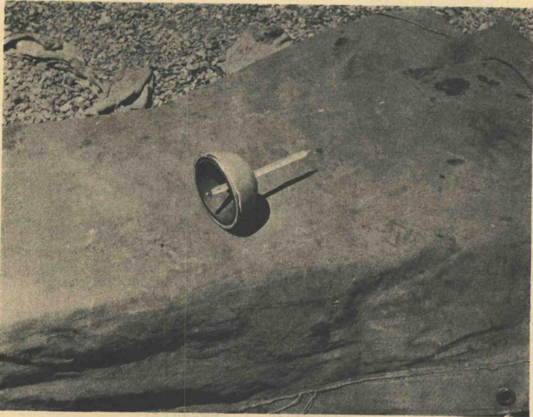
Figure 3. Bulb and Thermometer Used in Observing Pavement Surface Temperatures
