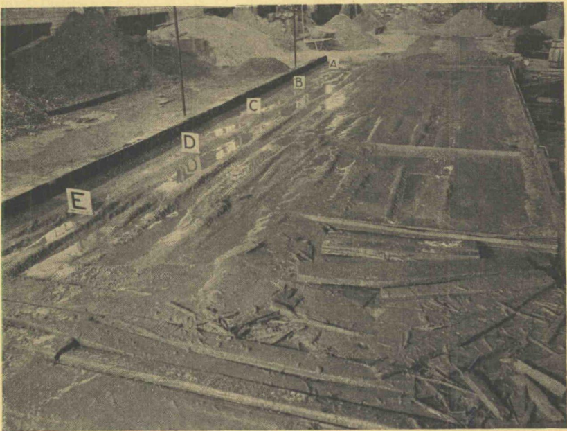
Figure 8. Five Hours of Wet Traffic Test on Indoor Test Road.
