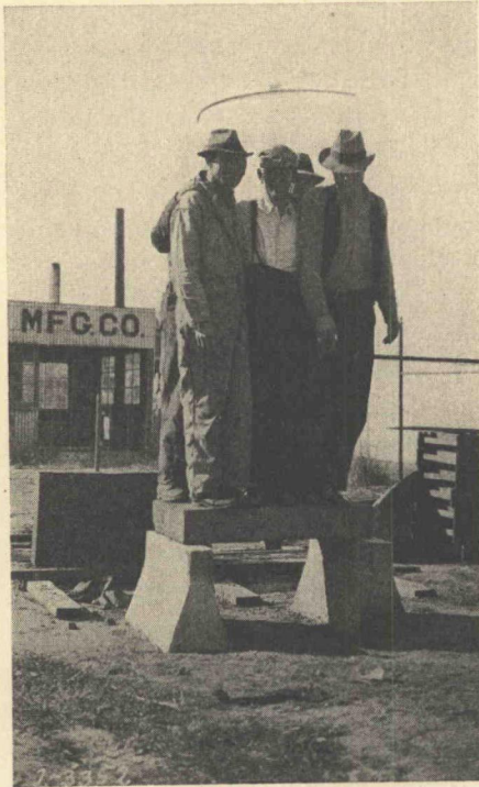
Figure 1. The beam supporting the men in this photo is a stabilized sundried adobe brick approximately 5" in thickness and stabilized by methods herein described. The beam was finally broken under a 1150 lb. dead load applied at the center.
