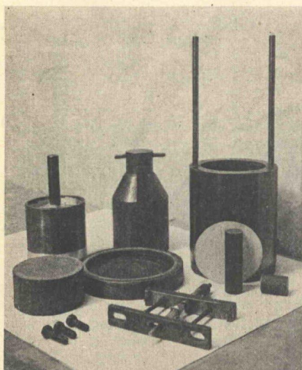
Figure 3. View of unassembled mold (showing compacting piston, "pressure pad," measuring device, filter paper, and soil pat) used in making swell tests in molds.
