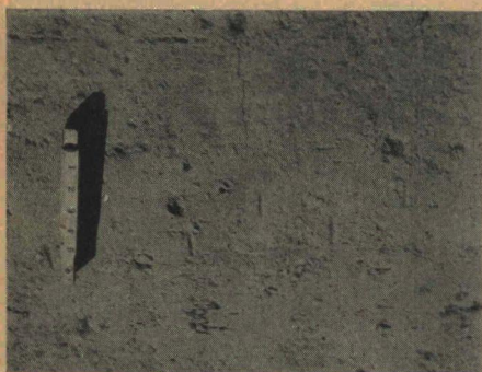
Figure 3. Close-up of surface of 8 per cent cement soil-cement mixed-in-place base after 7 days of cover with Sisalkraft paper. Note only very slight incipient cracking of surface.
