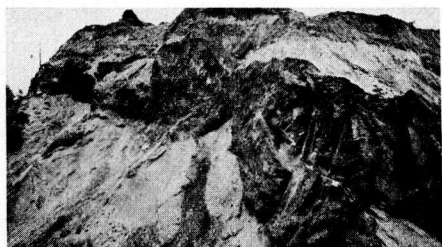
Figure 2. Sudden Changes in Soil Texture Exposed in Cuts through Morainic Areas. Such variations in texture favor differential heaving which in turn is responsible for rough riding and broken pavement. Michigan.
