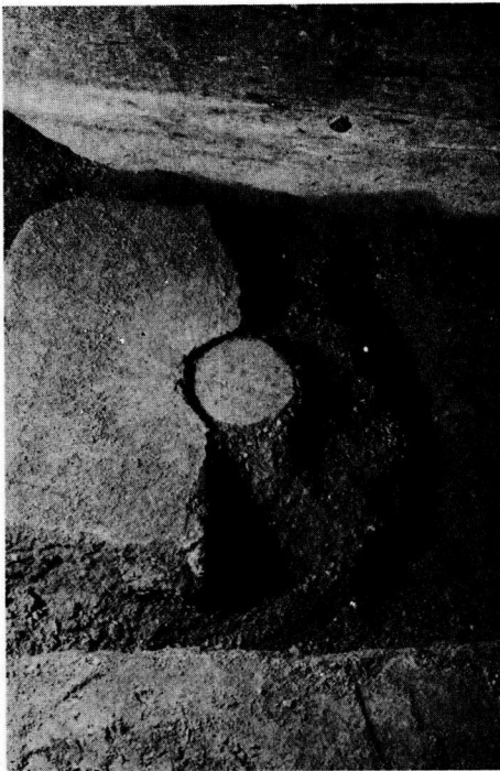
Figure 5. Appearance of screenings layer after making load-indentation test; circular bearing block, 10 sq. in. in area. Note the surface along which shearing action occurred during the test. Through the underlying cone the load is carried to the subgrade.
