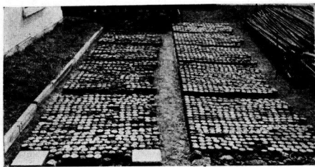
Figure 10. Wet-dry and freeze-thaw soil-cement specimens are stored outdoors at Elmhurst, Ill., after 12 cycles of laboratory testing.
