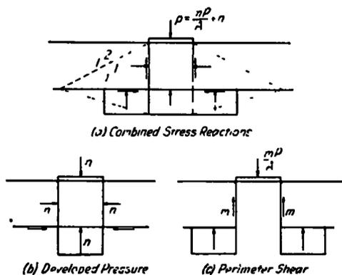
Figure 2. Stress Reactions in the Linear Equation for Bearing Capacity
