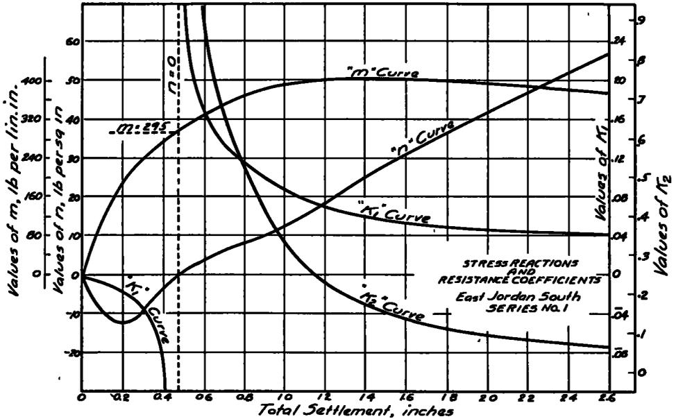
Figure 7. Analysis by Solution of Linear Equations at Equal Settlements
