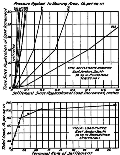
Figure 8. Typical Yield Value Analysis for a Flexible Surface
