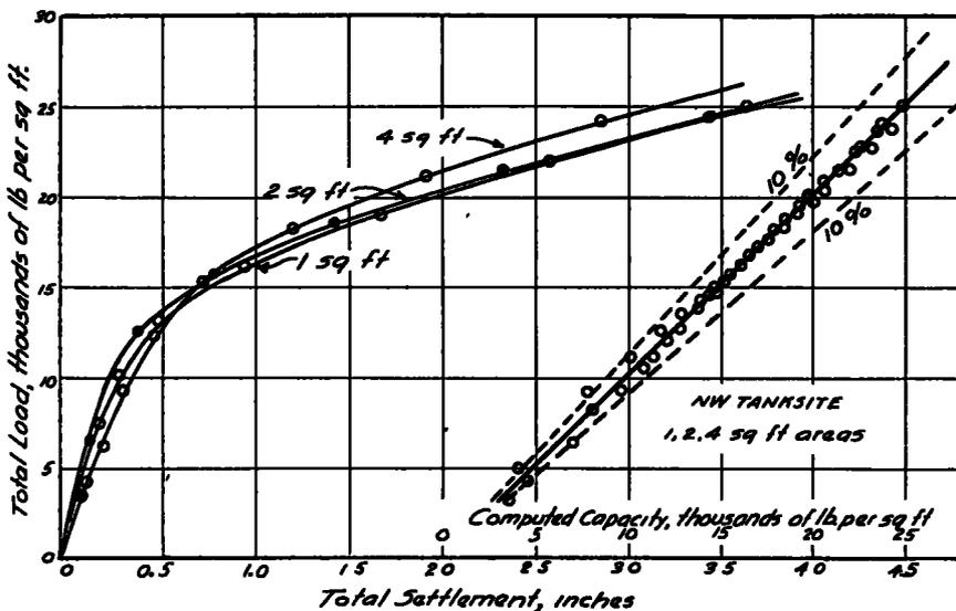
Figure 3 Corrected Load-Settlement Diagrams
