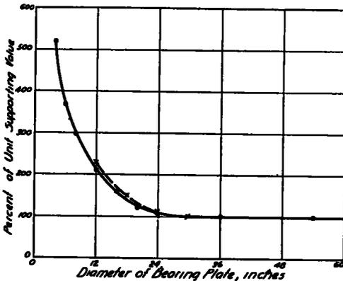
Figure 2. Relation Between Bearing Plate Diameter and Supporting Value of Soil.
