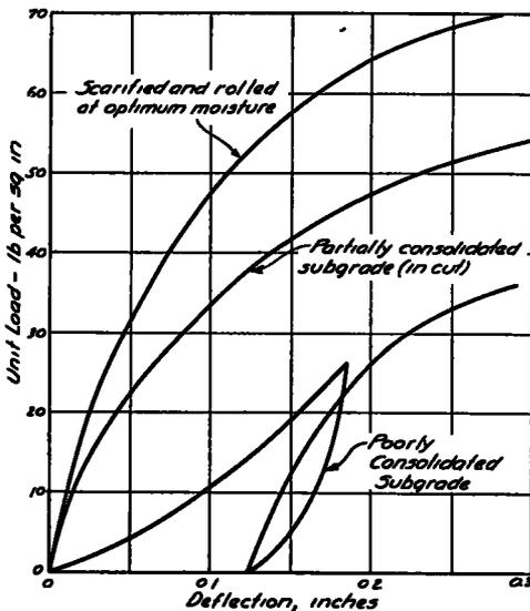
Figure 5. Effect of Subgrade Compaction
