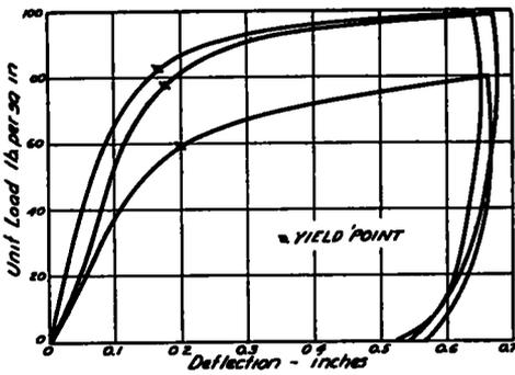
Figure 3. Comparative Test Data. Surface, Base Course and Subgrade
