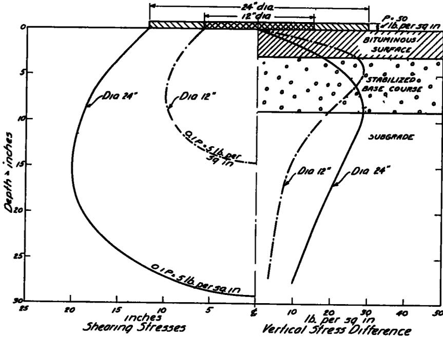
Figure 1. Effect of Increased Bearing Area on Subgrade Stresses
