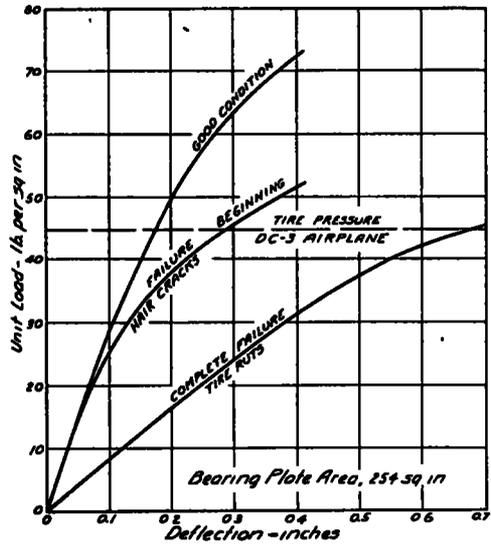
Figure 4. Condition Survey, Flexible Pavement at Commercial Airfield
