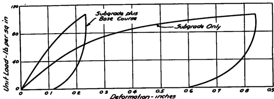
Figure 6. Subgrade and Base Course Bearing Tests
