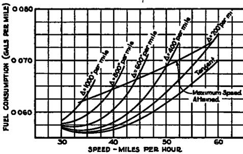
Figure 6. Fuel Consumption of 1937 Buick at 200-Deg. Increments of Central Angle Per Mile on Sections Constructed to New Alignment Standards.
