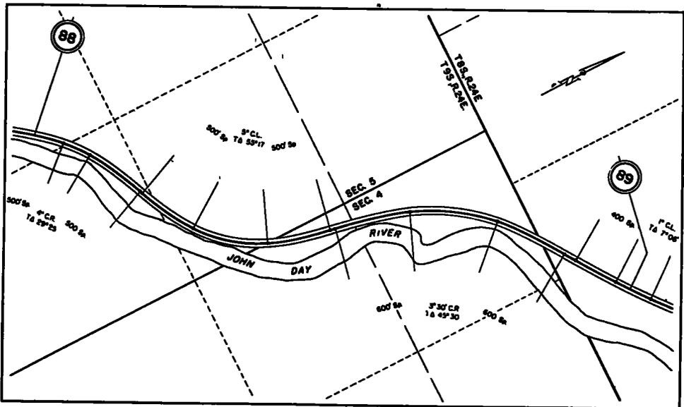
Figure 2. New Standard Alignment Test Section M.P. 88 to M.P. 89 on Ore. 19 North of Spray, Length of Section 1 Mile, Total Central Angle Per Mile=130 Degrees
