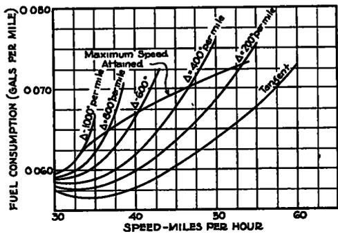
Figure 7. Fuel Consumption of 1937 Buick at 200-Deg. Increments of Total Central Angle Per Mile. Tests on Sections Having Old Alignment Standards.
