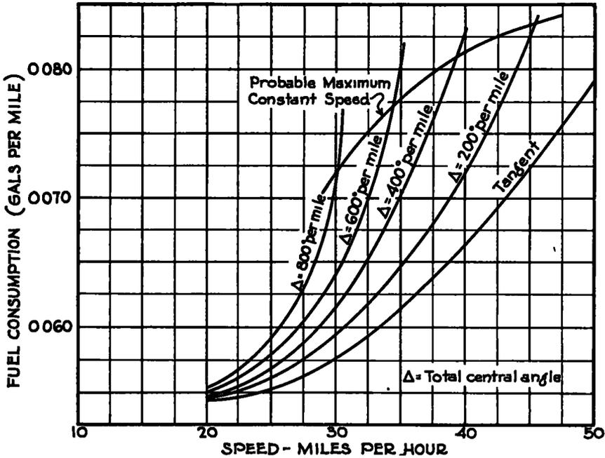
Figure 8. Fuel Consumption of 1939 Chevrolet Dump Truck at 200-Deg. Increments to 800-Deg. of Central Angle
