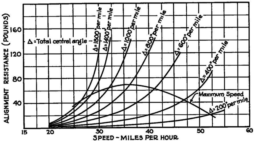
Figure 11. Average Effective Alignment Resistance Plotted at 200-Deg. Increments of Total Central Angle Per Mile, 1938 Ford Sedan
