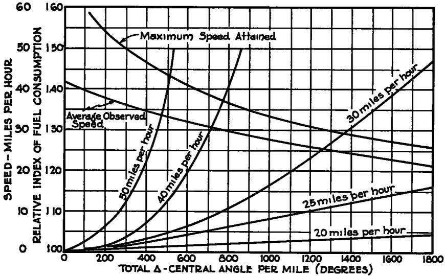
Figure 4. Relative Indices of Fuel Consumption and Maximum Constant Speed Attained on Each Test Section as a Function of Total Central Angle Per Mile (1938 Ford Sedan—Old Alignment Standards).
