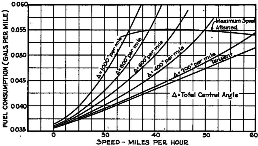
Figure 5. Fuel Consumption of 1938 Ford Sedan on Curved Alignment Shown in Increments of 200 Degrees of Central Angle Per Mile. Developed from Tests on Sections Constructed to Modern Alignment Standards.
