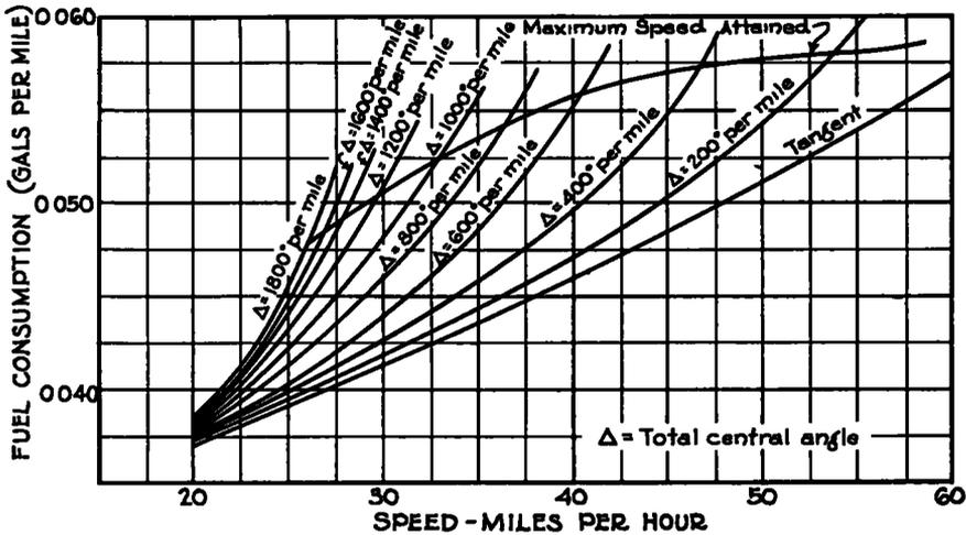
Figure 3. Fuel Consumption of 1938 Ford Sedan on Curved Alignment Shown in Increments of 200 Degrees of Central Angle Per Mile. Data Developed from Tests on Sections Constructed to Relatively Old Alignment Standards.
