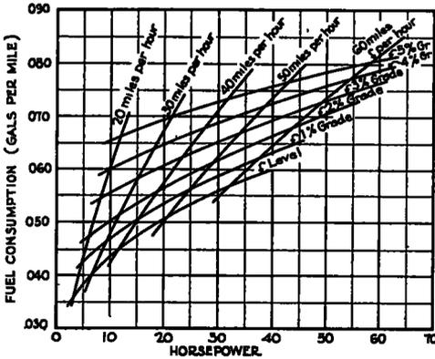
Figure 9. Fuel Consumption Vs. Horsepower for 1938 Ford Sedan
