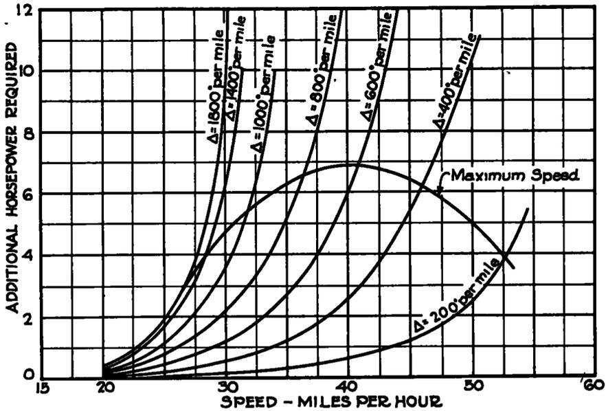
Figure 10. Horsepower Required to Overcome Alignment Resistance at 200-Deg. Increments of Total Central Angle Per Mile, 1938 Ford Sedan
