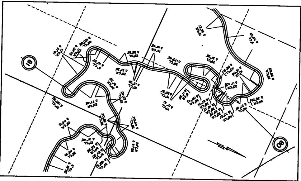
Figure 1. Old Standard Alignment Test Section M.P. 80 to M.P. 81, Upper Columbia River Highway, Length of Section 1 Mile, Total Central Angle Per Mile=1027 Degrees.
