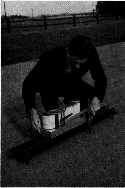
Figure 10. Road Profilometer Used to Measure Surface Texture
