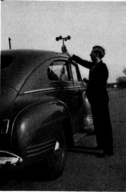
Figure 7. Four-Cup Anemometer Used to Measure Wind Velocity
