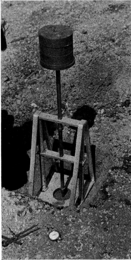
Figure 7. Apparatus for Cone Bearing Test
