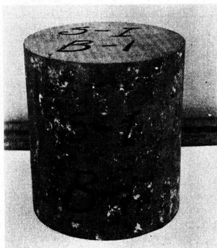
Figure 11. District 15 soil specimen before it was loaded to failure in the machine shown in Figure 16. The specimen had been dried to constant weight at 100 F., the ends ground smooth and parallel and the volume computed. The average diameter was 3.585 in., height 3.973 in., and the density was 124.6 lb. per cu. ft. The rupture load was 1700 lb. per sq. in. and the deformation at the time of rupture was 0.056 in.
