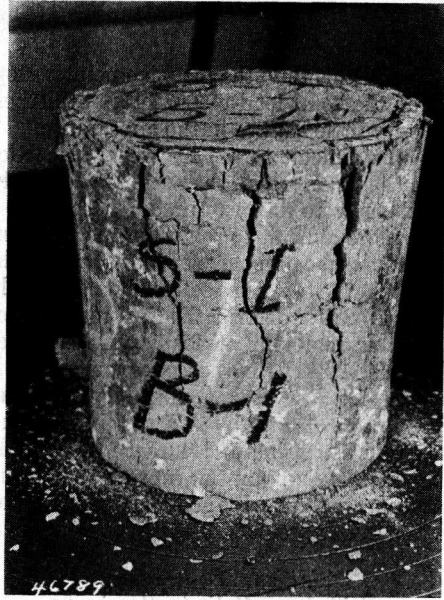
Figure 14. Close-up of specimen shown in Figure 13 after the testing machine pointer stopped at 6,475 lb. and machine continued to run. The loose outside broken pieces of soil then were scratched down.
