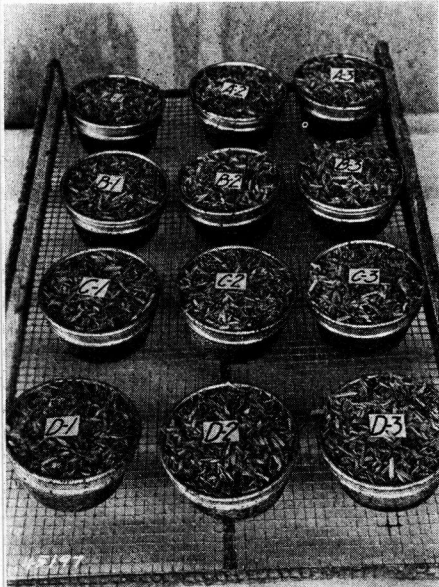
Figure 2. Soil specimens packed in damp sawdust for slowly raising the moisture content of the specimens.
