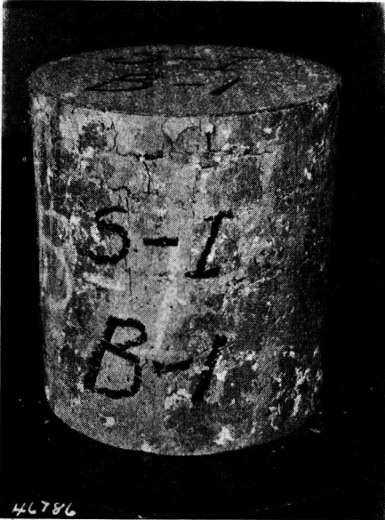
Figure 13. Close-up of specimen immediately after rupture at 17,150 lb. Platen of testing machine raised for this picture. Load then slowly re-applied until pointer stopped at 10,350 lb. Platen again was raised but no change in appearance of specimen could be seen. Load again was slowly applied until pointer stopped at 6,475 lb. No difference in appearance of specimen at that time.
