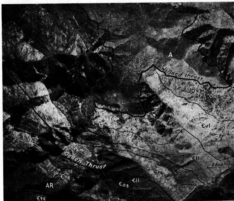
Figure 7. Vertical aerial photograph of an area in the Wasatch Mountains northeast of Ogden, Utah, upon which the contacts of the various rock formations have been inked in. AR, Archean granite and gneiss; A, Proterozoic quartzites and phyllites; C + q, Cambrian quartzite; Cos, Cambrian shale; ClI, Lower Cambrian limestones; Cul, Upper Cambrian limestones. Courtesy U.S. Forest Service
