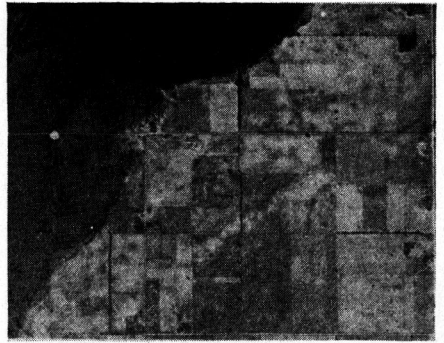
Figure 9. Airphoto showing the contrast in color tones existing between light colored (well drained) terrace soils and dark colored (poorly drained) alluvial soils. (Wabash Valley, Indiana.)
