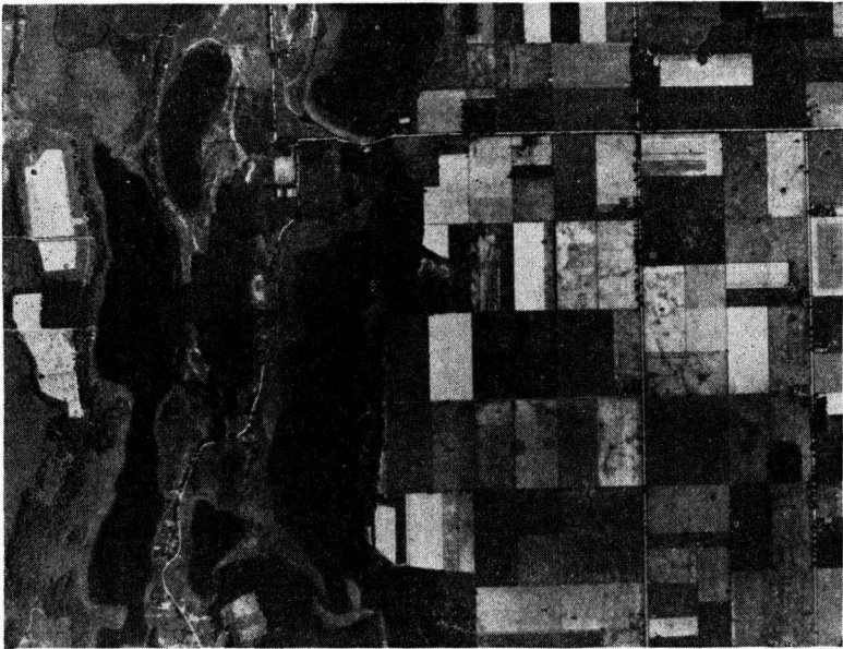
Figure 19. Airphoto Pattern of a Glacial Outwash Plain in Elkhart County, Indiana. This contains the elements of light color tone, mottling effect, and glacial lakes.
