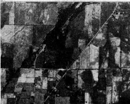
Figure 26. This esker near Indianapolis, Indiana is partially outlined by a heavy timber cover. The esker is crescent shaped and over a mile in length.
