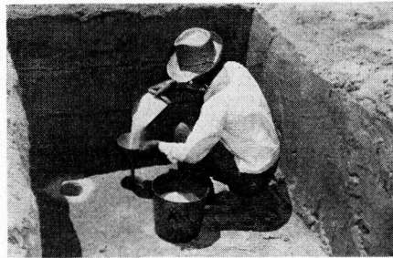
Figure 9. Field Density Determination by Sand Displacement Method.
