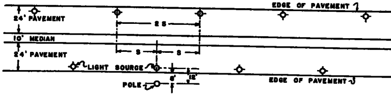
Figure 1. Freeway Design No. 1 Showing lighting layout for which cost estimates are provided. Lamp spacing (S) is shown in Table 1 for different lamp sizes and luminaires.
