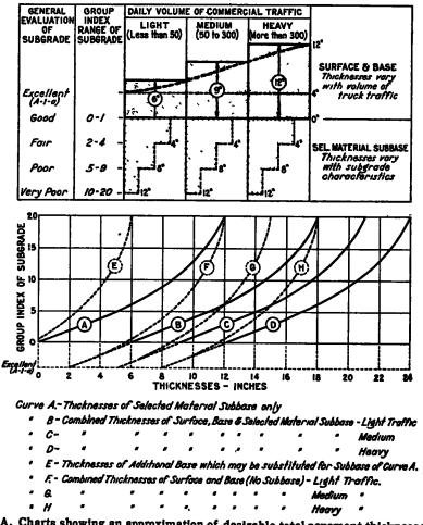
Figure A. Charts showing an approximation of desirable total pavement thicknesses (surface, base and subbase) based on truck traffic volume and group index of subgrade. (See discussion for Explanations, Assumptions and Exceptions.)
