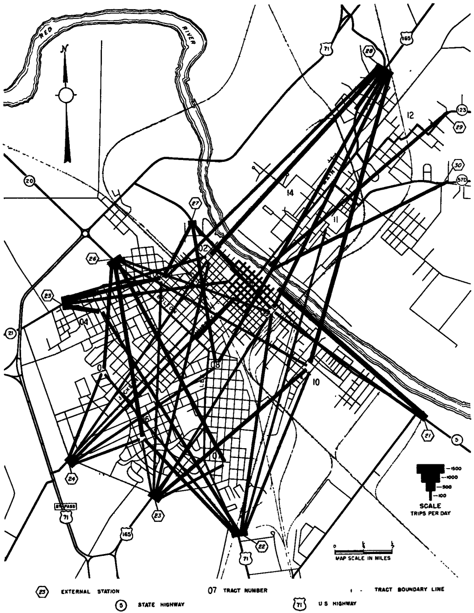
Figure 13. Internal and External Automobile Trips Combined, Volume Range of 100 to 249 in Alexandria, La.
