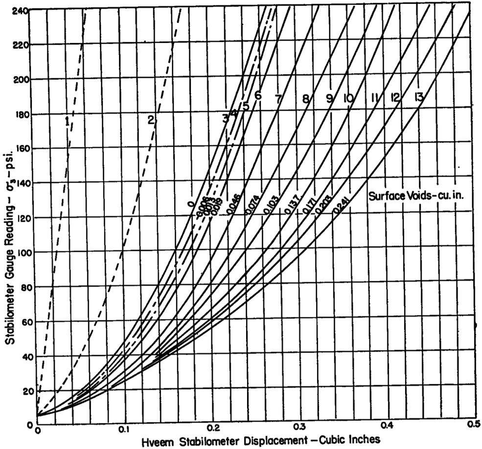
rigid system with no occluded air, respectively. They are drawn from data given in Mr. Hveem's instructions for the care and use of the stabilometer. Curve 1 is drawn straight thru the point given in Mr. Hveem's data on the assumption that the gauge reading is proportional to the volume deformation causing it if the system is rigid, and curve 2 is drawn
