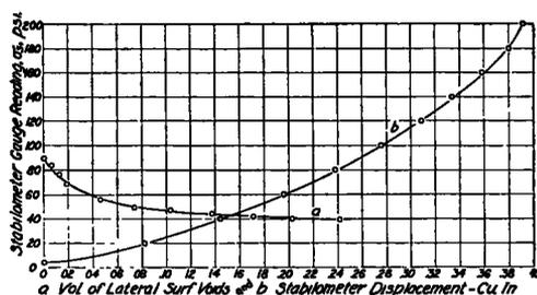
Figure 5. Vertical Stress-Vertical Deformation Curves for (a) Asphaltic Concrete Specimen R-A<sub>6</sub>-R<sub>2</sub>-12-3(1), (I.P. No. 11) in Confined Compression and (b) Specimen X-18 (S.I. No. 7) in Unconfined Compression
