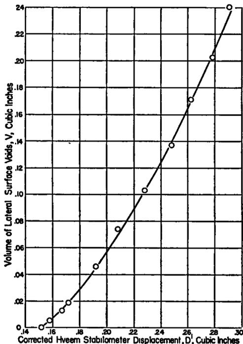
Figure 2. Relation between Volume of Lateral Surface Voids and Hveem Displacement on Brass Dummy Specimen
