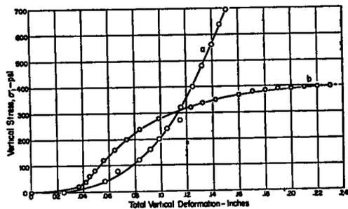
Figure 3. Relation between Stabilometer Gauge Reading and (a) Volume of Lateral Surface Voids at a Constant Stabilometer Displacement of 0.152 Cu. In. and (b) Stabilometer Displacement in Cubic Inches at a Constant Volume of Surface Voids (0.152 Cu. In.)
