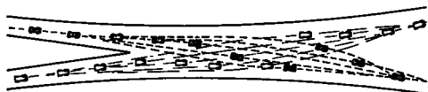
Figure 9. Note: Spacing of Vehicles on Approach Roadways Based on Speed of 20 MPH With Time Gap Between Vehicles of 1.1 Seconds
