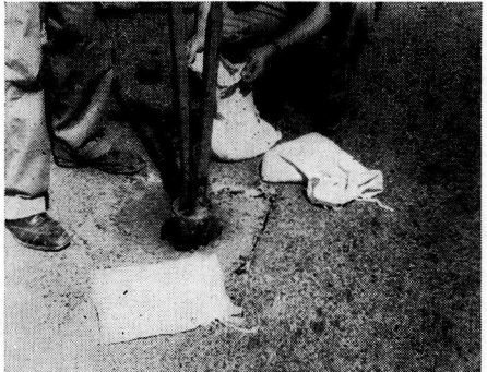
Figure 7. Taking 15-lb. Sample of Soil for Laboratory Tests. This picture shows sampling of the base material.
