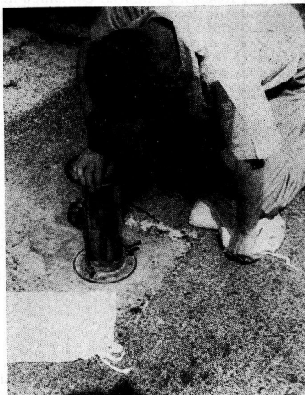
Figure 3. Taking "Zero" Reading with Rubber Balloon Density Apparatus
