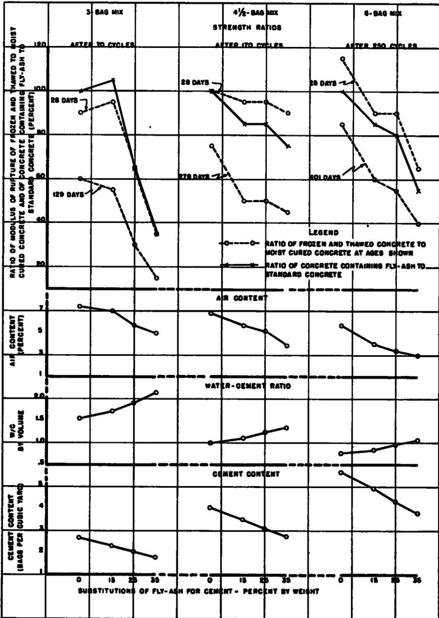
Figure 2. Cement Content, Water-Cement Ratio, Air Content and Resistance to Freezing and Thawing of Six-Inch Slump Concrete Containing Fly-Ash
