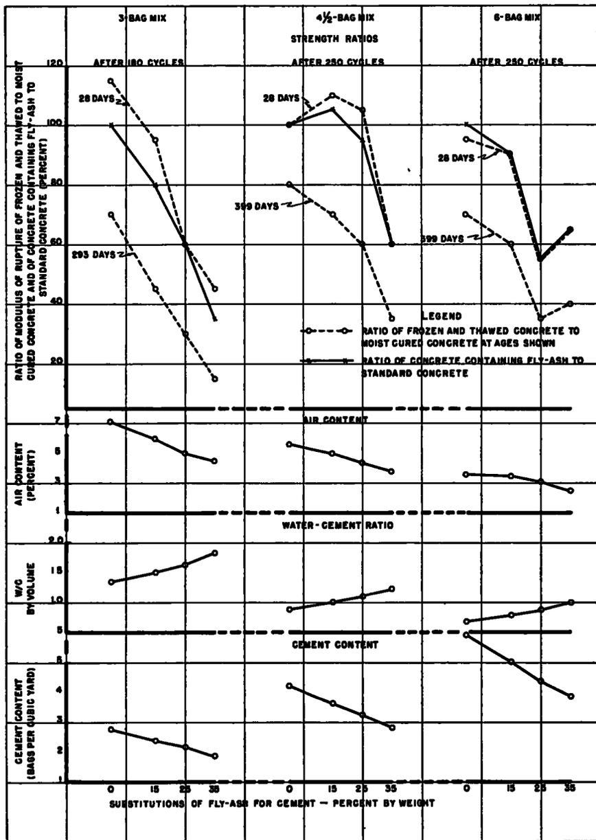
Figure 1. Cement Content, Water-Cement Ratio, Air Content and Resistance to Freezing and Thawing of Six-Inch Slump Concrete Containing Fly-Ash
