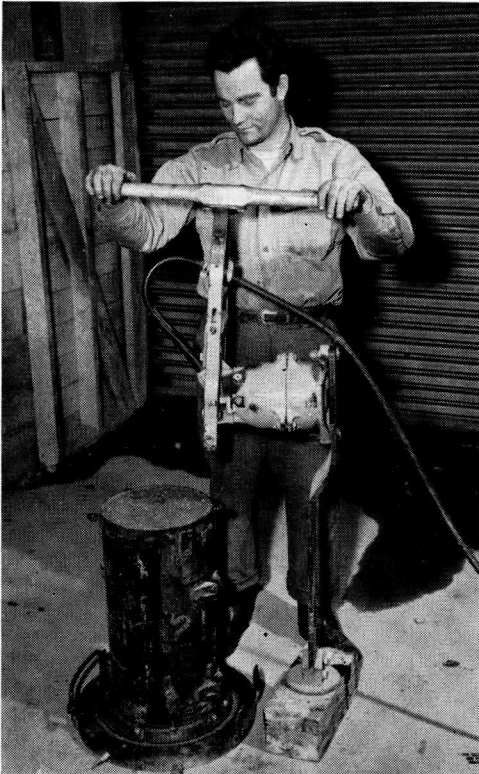
Figure 3. Vibratory tie tamper: used for compaction of triaxial samples.
