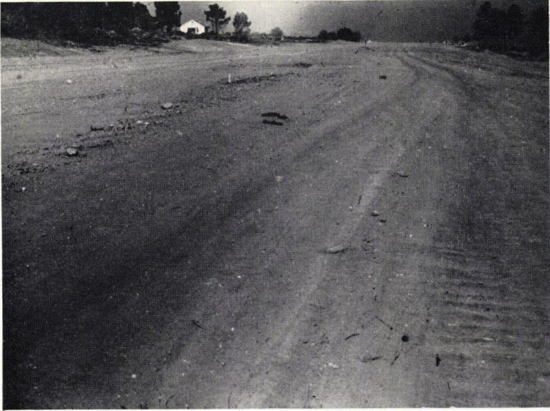
Figure 1. Soil which by old rating system would require treatment. LL = 54, PI = 17; minus No. 200 = 62 percent; total volume change, 8 percent; maximum density, 95 lb. per cu. ft.
