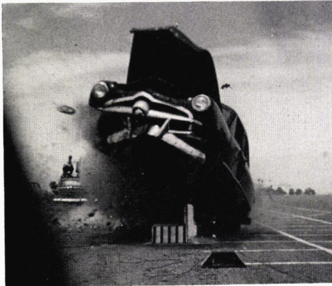
Figure 1. Test collision shortly after initial contact. Note recording movie camera in foreground.
