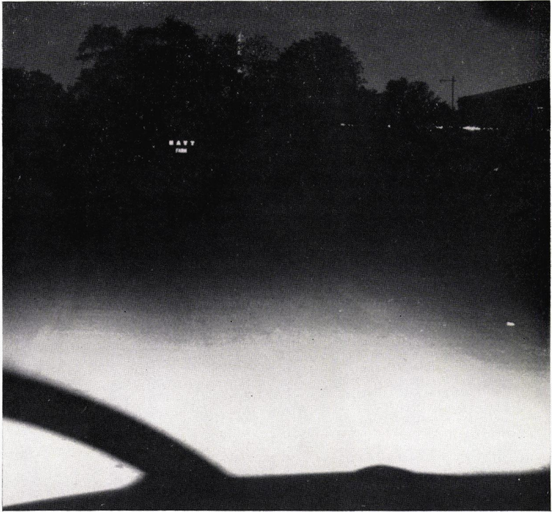
Figure 4. Appearance of sign panel from a distance of 600 feet.
