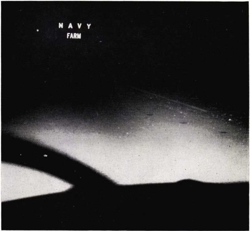
Figure 6. Appearance of sign panel from a distance of 200 feet.
