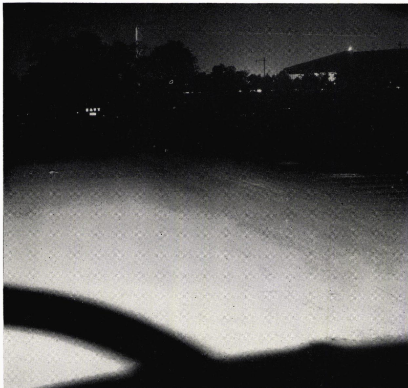
Figure 3. Appearance of sign panel from a distance of 800 feet.
