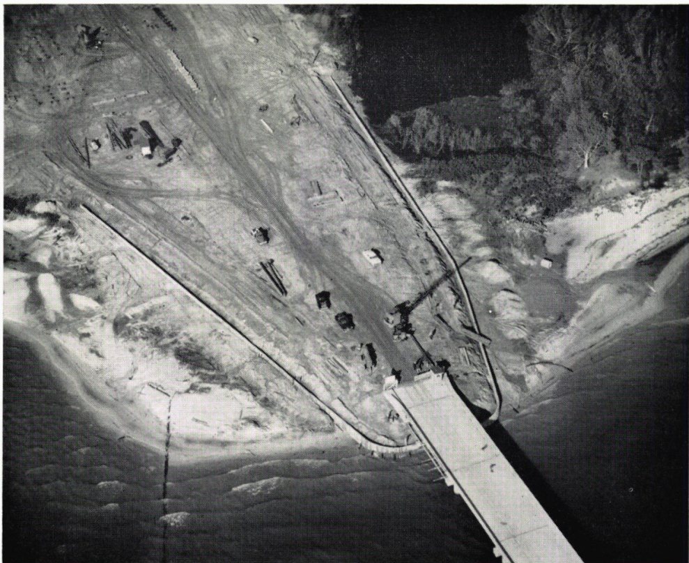
Figure 13. North plaza with surcharge removed and sea wall in place.
