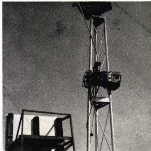
Figure 2. Camera mounted on 30-ft television tower with auxiliary tower for personnel.
