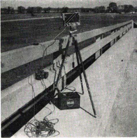
Figure 3. Tripod-mounted camera on overhead structure.
