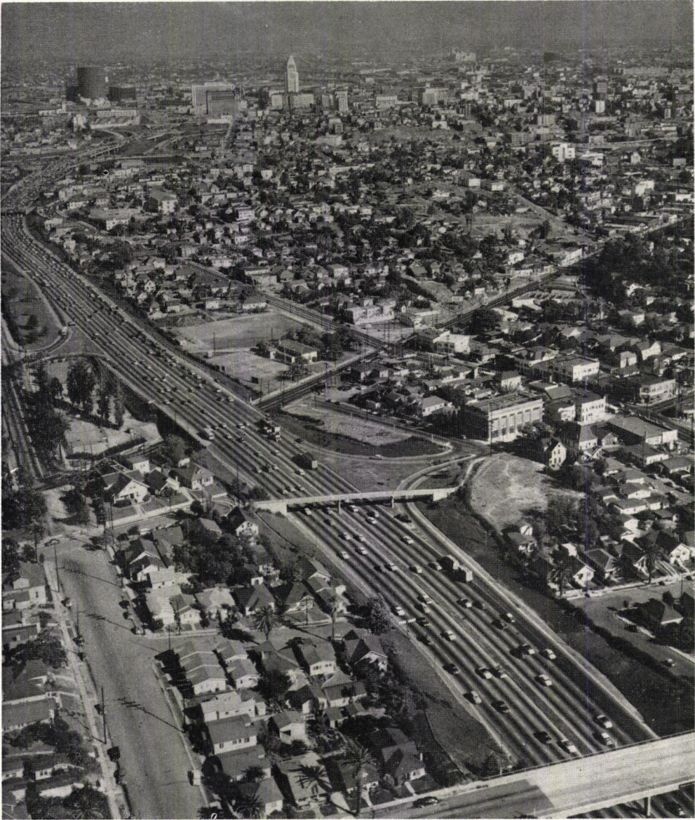
Figure 2. Hollywood Freeway looking southerly toward Los Angeles Civic Center. Alvarado SB on-ramp (Location 18) just north of Bonnie Brae Street Bridge in foreground. Belmont Avenue pedestrian separation in center and Edgeware Street Bridge (Location 11) in background. This section is considered a typical 8-lane freeway with respect to geometric conditions affecting traffic operation.
