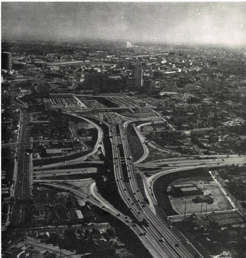
Figure 1. Hollywood Freeway looking southerly with the four-level traffic interchange in the foreground. Location 15 is at the merge in the foreground, Location 26 is at the merge of traffic going away in the center right, Location 37 is just past the second overcrossing in the center of the picture. This intersection handles 319,000 vehicles per day (25,500 in the peak hour, with 6,700 making left turns).
